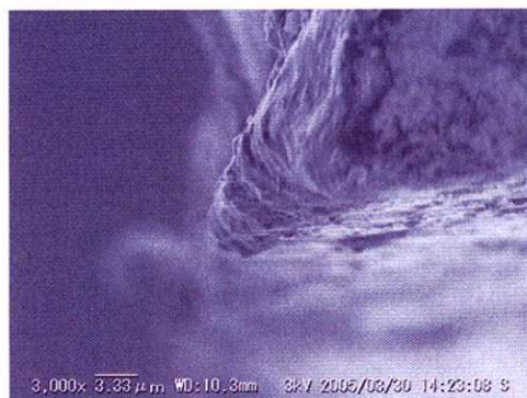
(c) Diamond tool, rake angle: 30deg.
