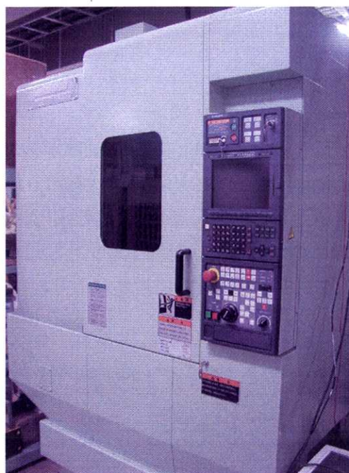
(b) Mori seiki, Accumill4000 (Max. spindle speed: 15,000 rpm)
