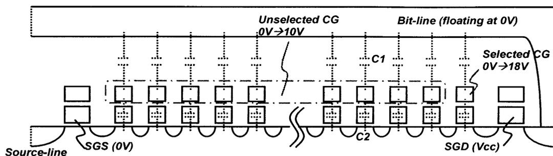
Fig. 6.14 Capacitive coupling noise between control gates and a bit-line. During the "0"-program, the bit-line is kept floating at 0V.
