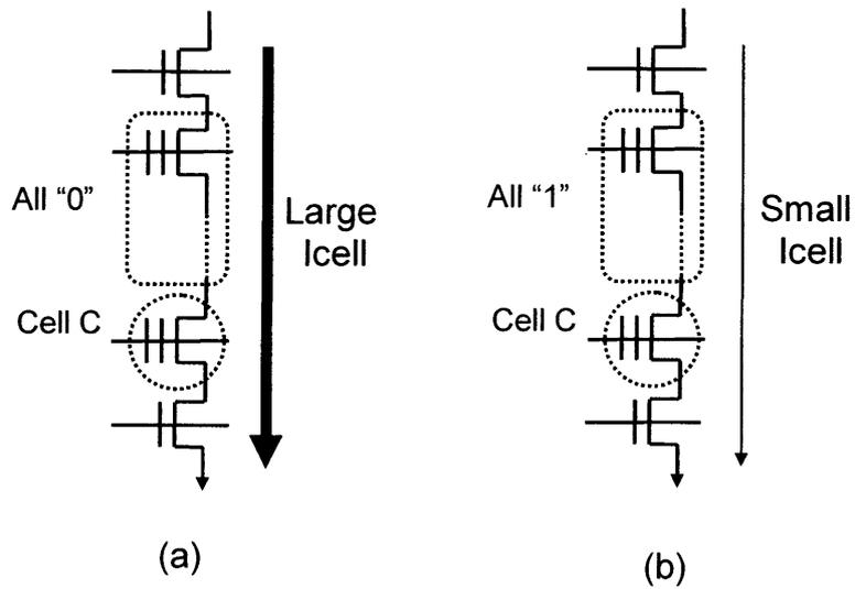
Fig.5.7 A model for the threshold voltage shift in the positive direction due to the source-line noise.
