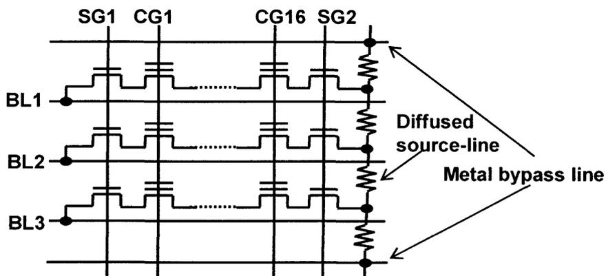
Fig.5.2 A NAND-type cell array. Each NAND cell unit shares sixteen control gates, two select gates, and a diffused source-line which is shunted with metal bypass lines. As the number of metal bypass lines increases, the source-line resistance decreases with a drawback of a cell area overhead.
