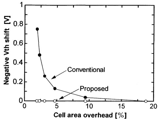
Fig.5.6 Calculated threshold voltage shift in the negative direction due to the source-line noise.
