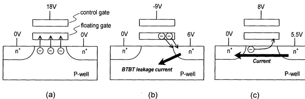
Fig. 6.4 (a) Channel FN-tunneling programming. The programming current is a few pico-amperes and is very small [12-15].
