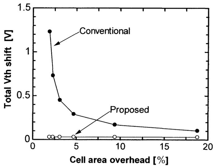
Fig.5.9 Calculated total threshold voltage shift due to the source-line noise.
