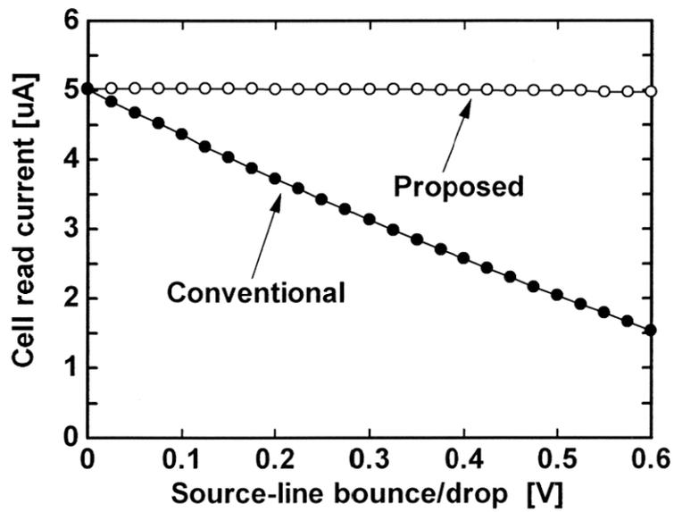
Fig.5.18 Measured cell read current change due to the source-line drop in the proposed cell and the source-line bounce in the conventional cell.
