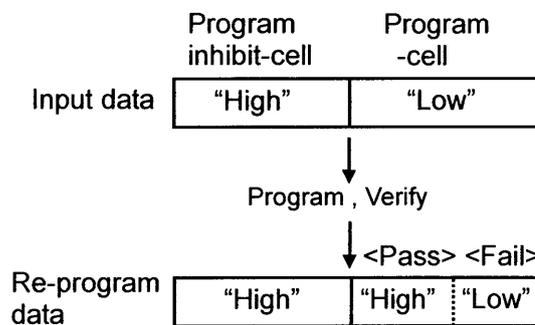
Fig.5.15 Program and re-program data stored at the page buffer node,  $N_{sense}$  during a programming and a program verify read.
