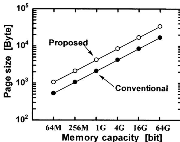
Fig. 6.12 Page size trend. The chip size of the proposed scheme is assumed to be the same as that of the conventional scheme.
