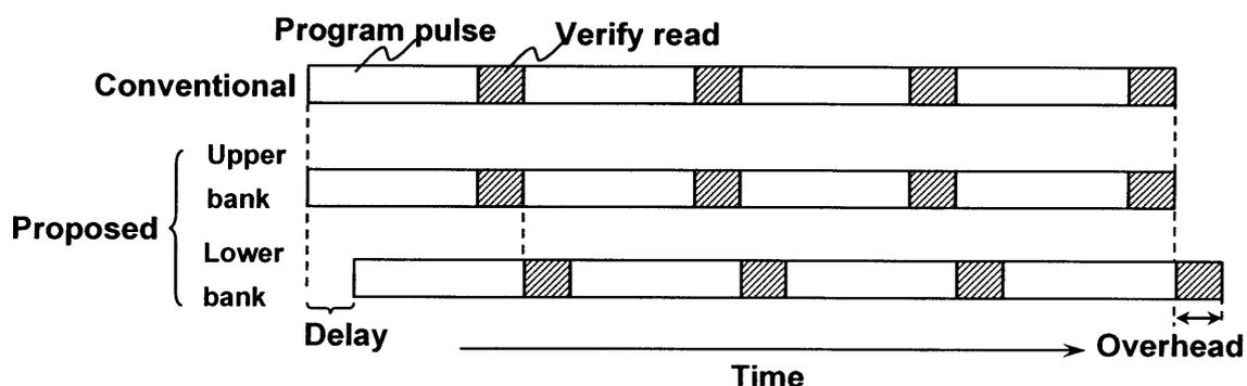
Fig. 6.11 Comparison of the conventional and the proposed program operations. The number of program and verify read cycles is assumed to be four.
