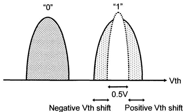
Fig.5.1 Schematic threshold voltage distribution. The threshold voltage distribution without array noise can be narrowed to 0.5V if the program voltage increment is 0.5V. Due to array noise, threshold voltages of memory cells shift in both positive and negative directions.
