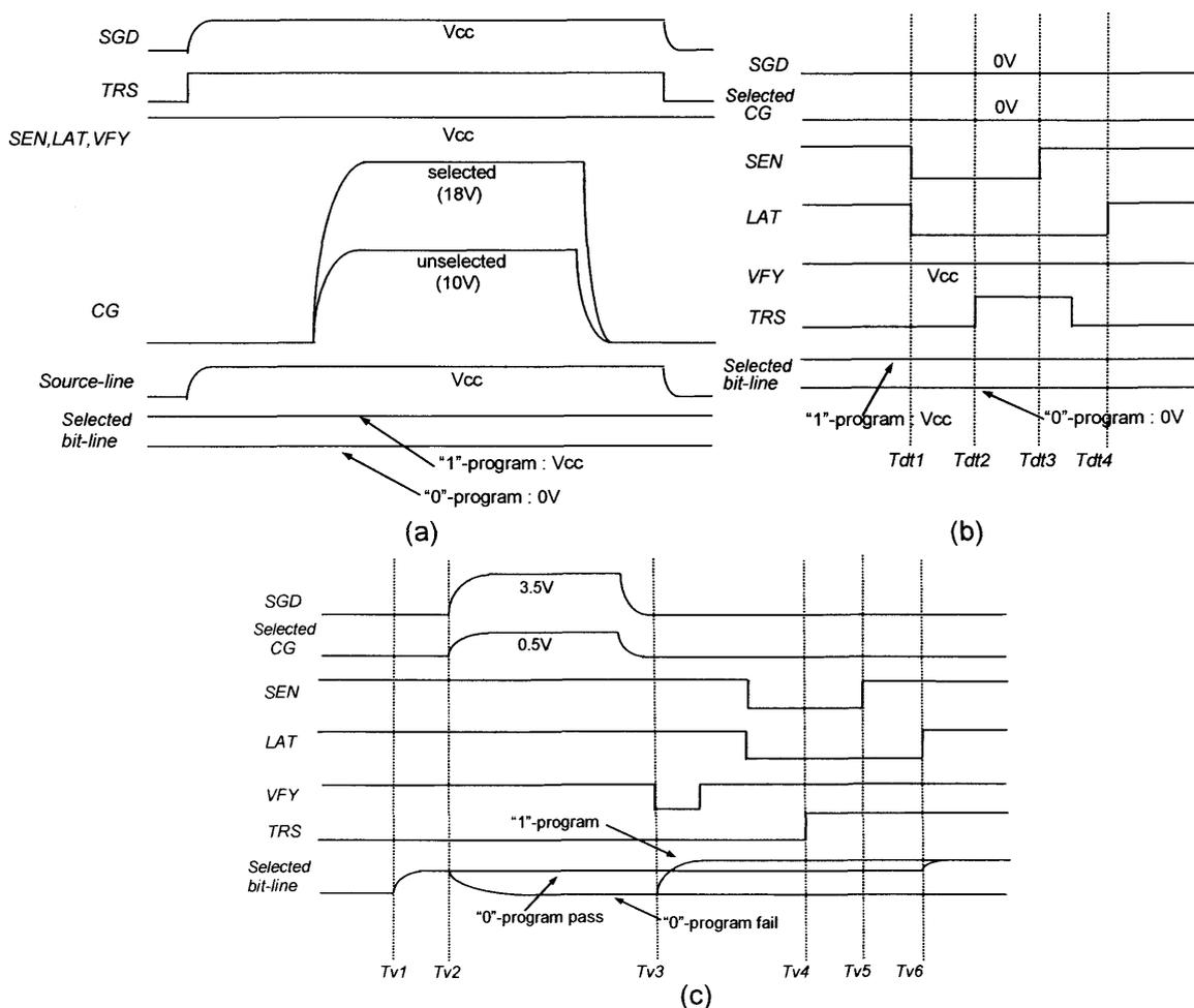
Fig. 6.10 Signal timing diagram. (a) Program pulse. (b) Data transfer from the bit-line to the page buffer. (c) Verify read operation.
