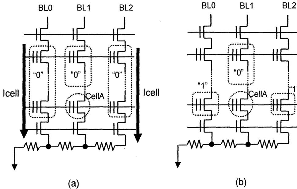
Fig.5.3 A model for the threshold voltage shift due to inter bit-line capacitive coupling noise.
