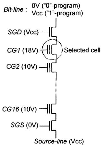
Fig. 6.1 Program operation of a NAND-type cell
