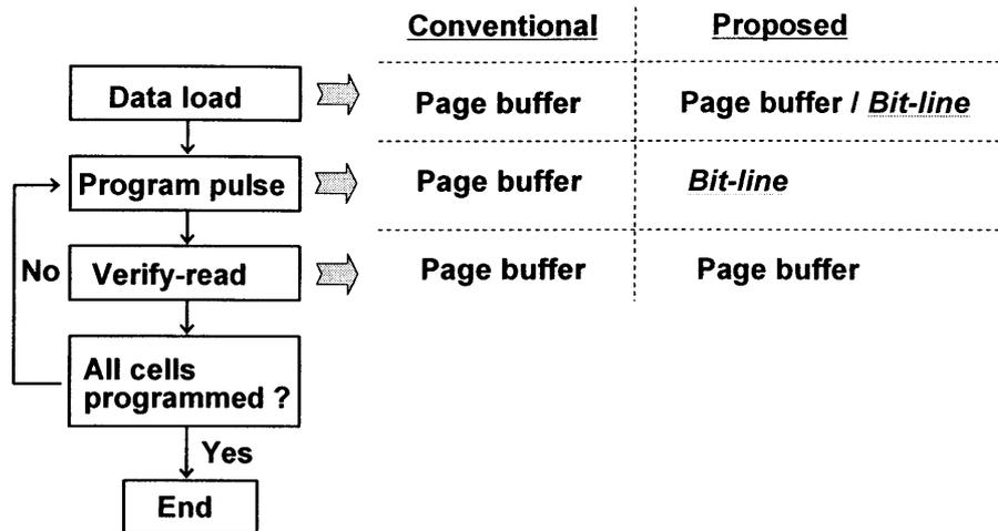
Fig. 6.3 Circuits storing the program data. In the conventional scheme, a page buffer stores the program data throughout the program operation. In the proposed scheme, a bit-line is used as a dynamic latch storing the program data.
