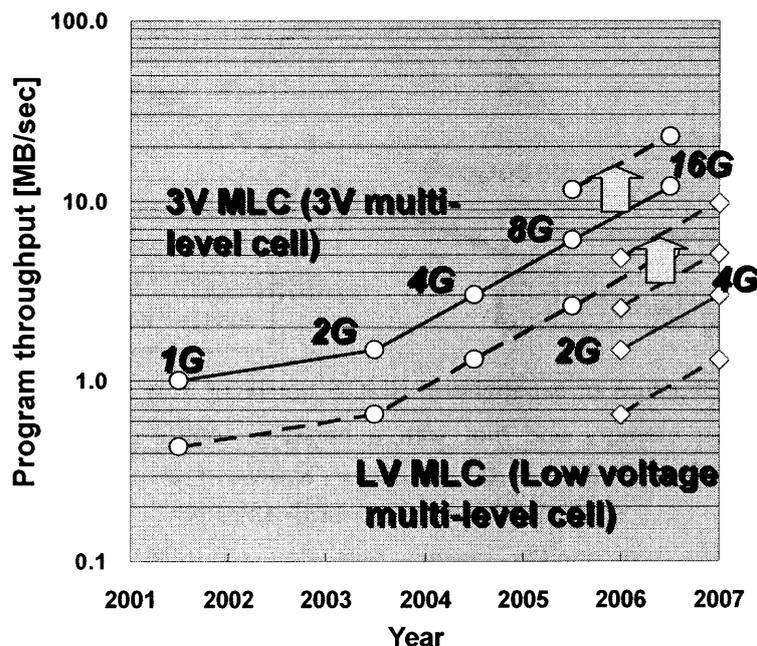
Fig.5.20 Program speed improvement with the low noise technology
