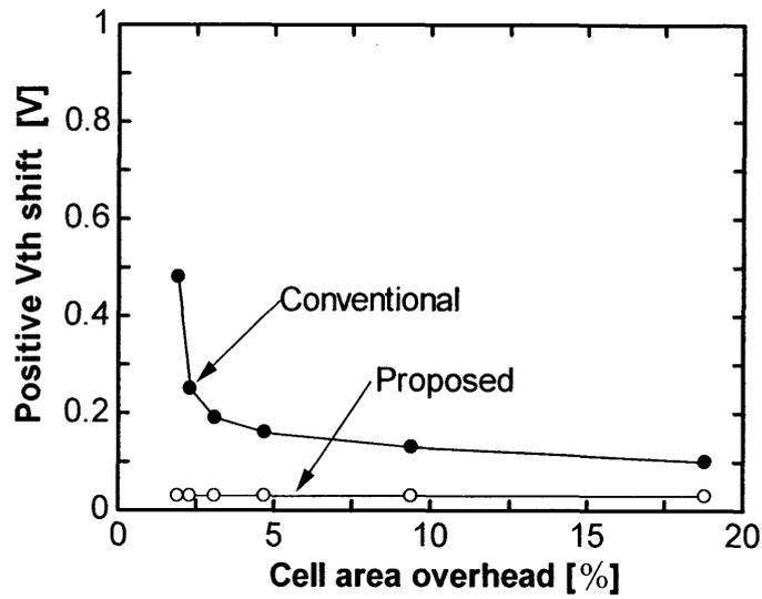
Fig.5.8 Calculated threshold voltage shift in the positive direction due to the source-line noise.
