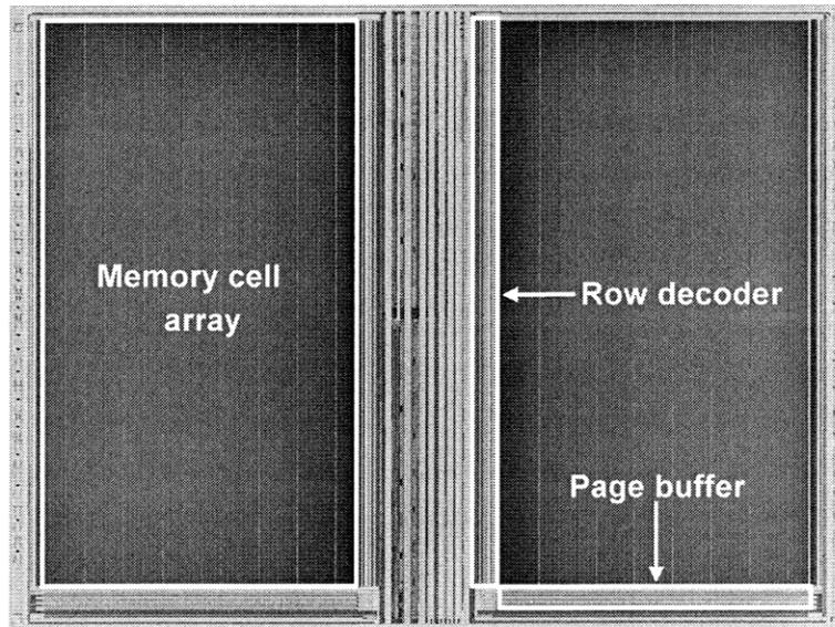
Fig.5.17 A micrograph of the proposed 256Mbit NAND flash memory chip.
