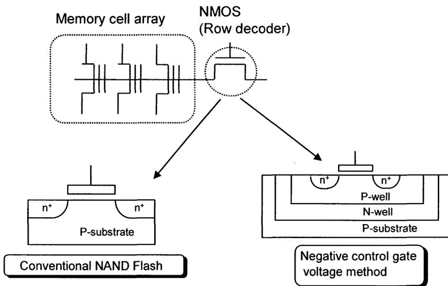
Fig.5.19 Structure of a peripheral NMOS transistor in a conventional NAND flash memory and that with a negative control gate voltage method.
