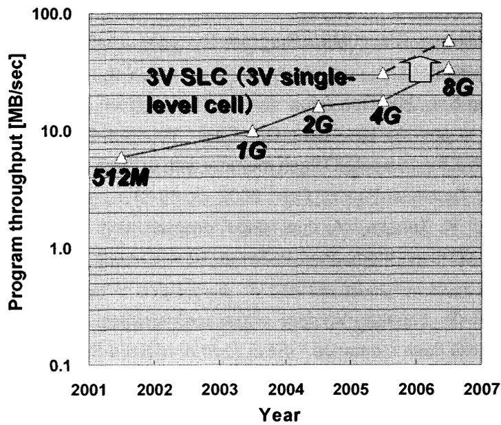
Fig.6.15 Program speed improvement with the parallel write technology
