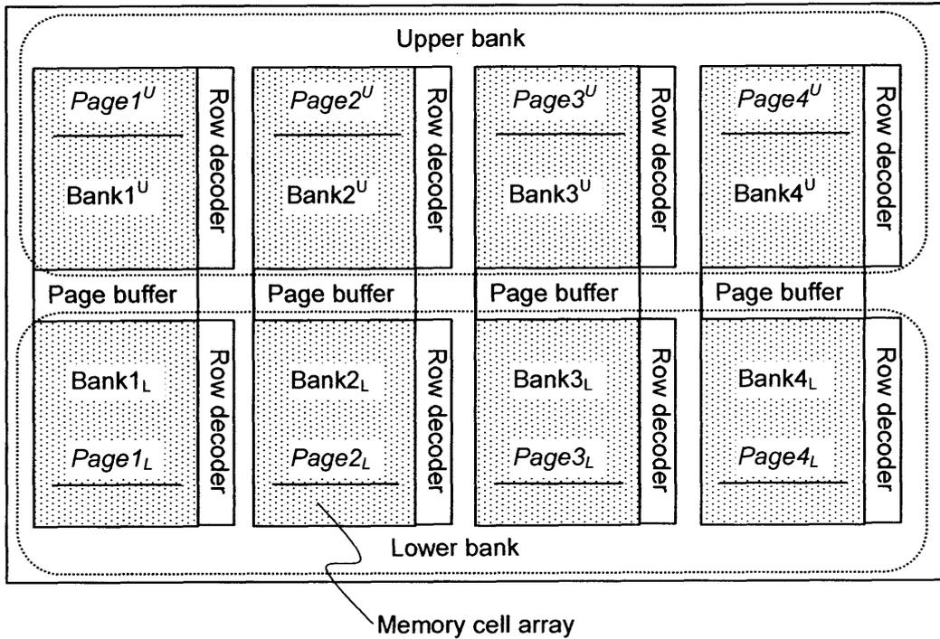
Fig. 6.5 A diagram of the proposed 1-Gbit NAND flash memory. Bank<sub>1,2,3,4</sub><sup>U</sup> compose the upper bank and the lower bank consists of Bank<sub>1,2,3,4</sub><sup>L</sup>. The page size of each bank is 4-kbit. The maximum page size is 32-kbit.
