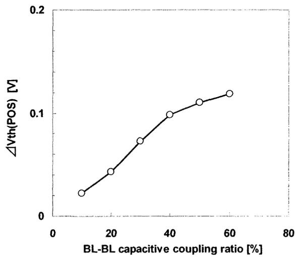
Fig.5.4 Calculated threshold voltage shift in the positive direction due to inter bit-line capacitive coupling noise.
