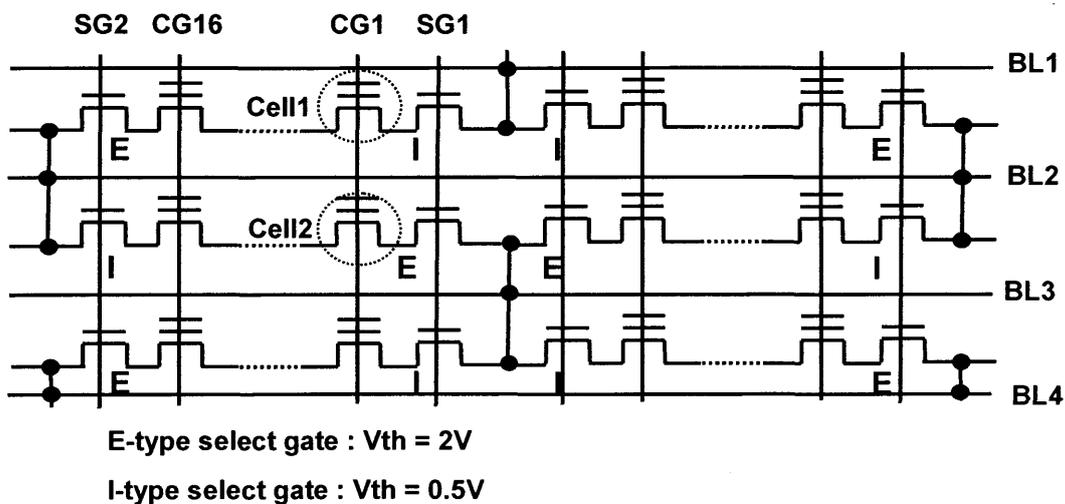
Fig.5.10 A double-level-Vth select gate array architecture. Each NAND cell unit is composed of an E-type select gate ( $V_{th}=2.0V$ ), an I-type select gate ( $V_{th}=0.5V$ ) and 16 memory cells.
