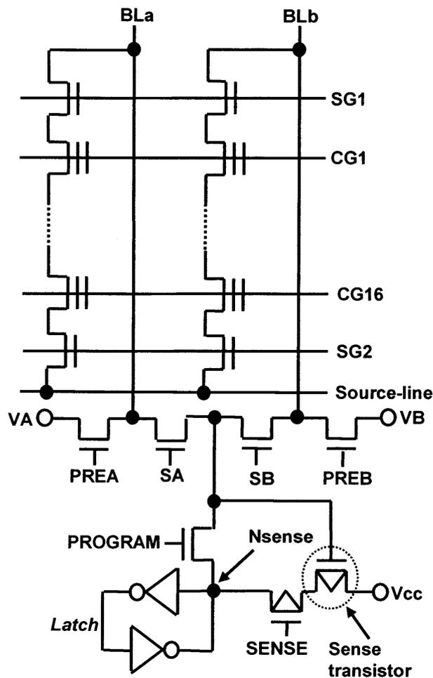
Fig.5.13 A simplified schematic diagram of the proposed PMOS drive page buffer.
