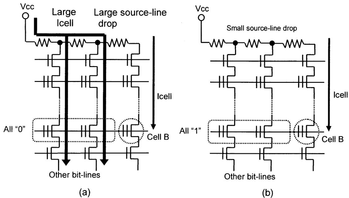
Fig.5.16 A model for the negative threshold voltage shift of the proposed cell due to source-line noise.
