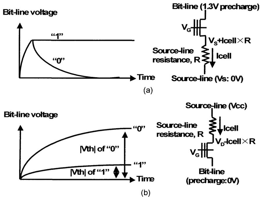
Fig.5.12 Comparison of the conventional (a) and the proposed (b) sensing methods.
