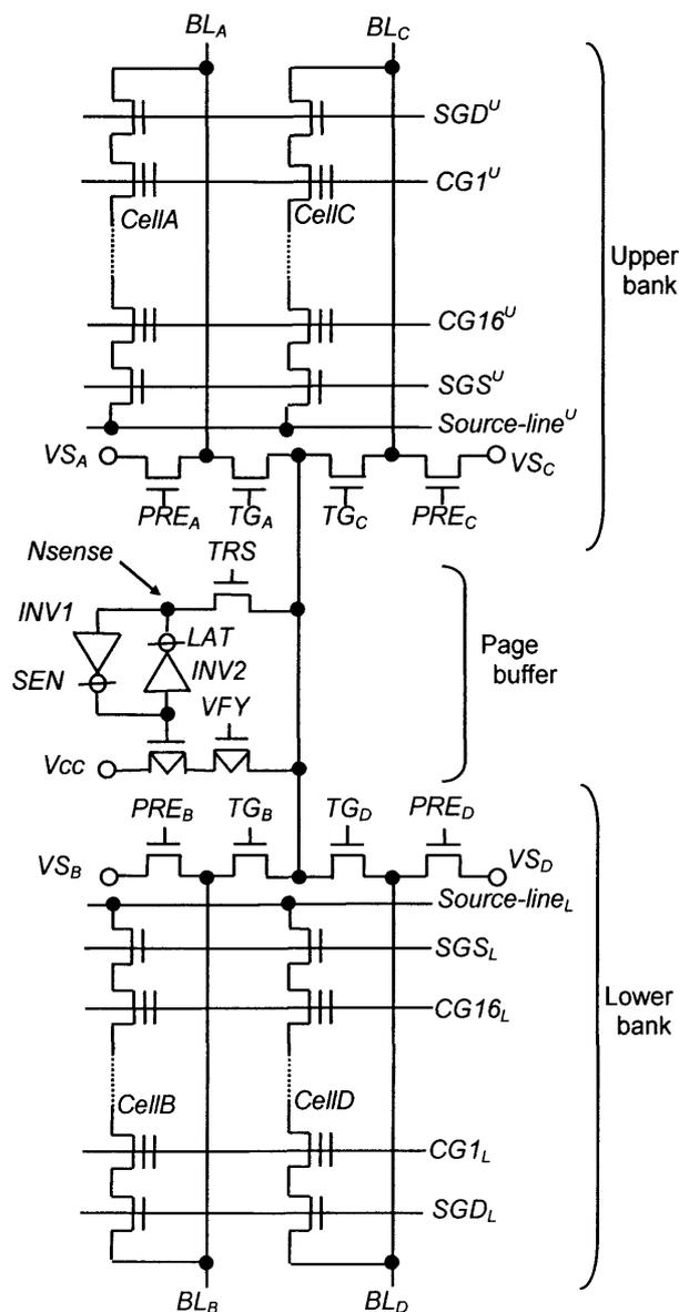
Fig. 6.8 Simplified schematic diagram of a proposed page buffer.
