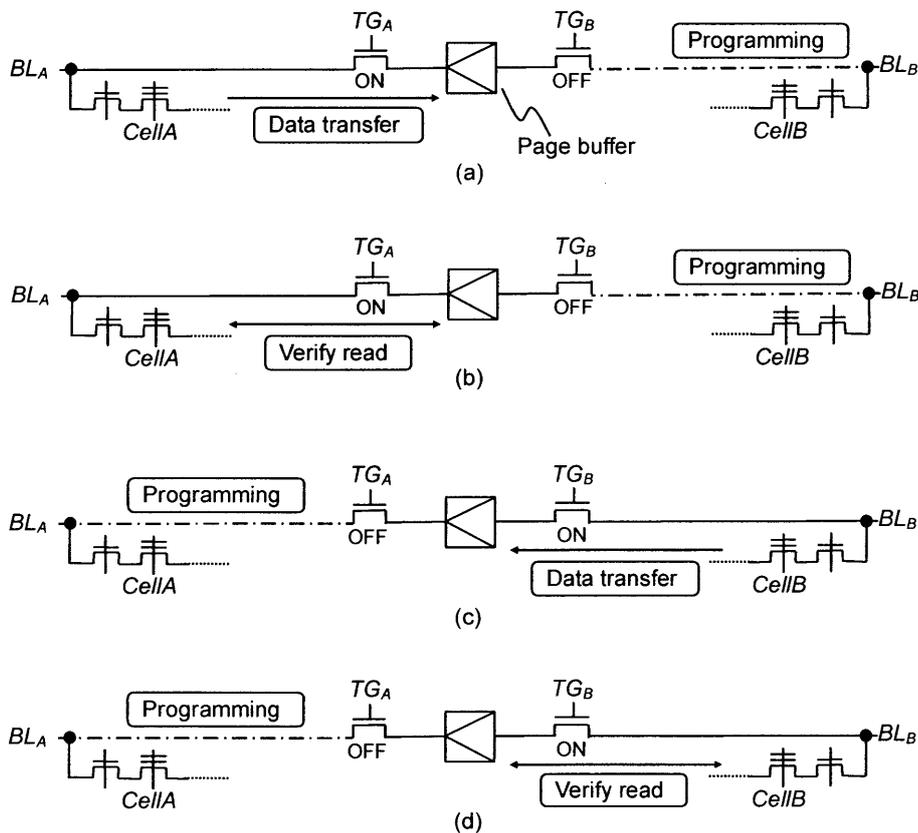
Fig. 6.2 Key operations of the proposed scheme.
