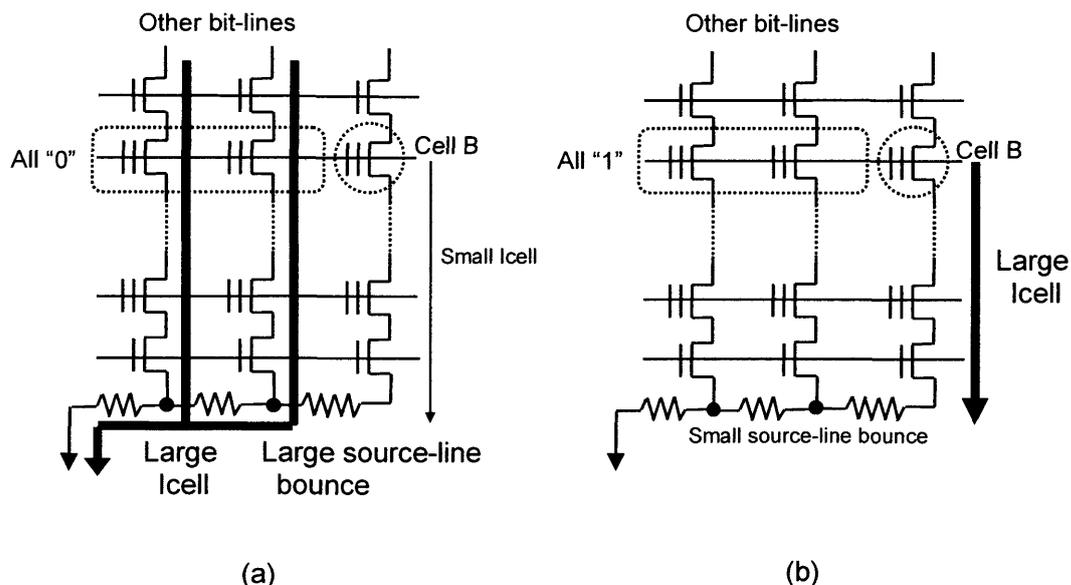
Fig.5.5 A model for the threshold voltage shift in the positive direction due to the source-line noise.
