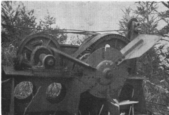
③ "Owase L-III" fan-governor, installed for a skyline crane.
