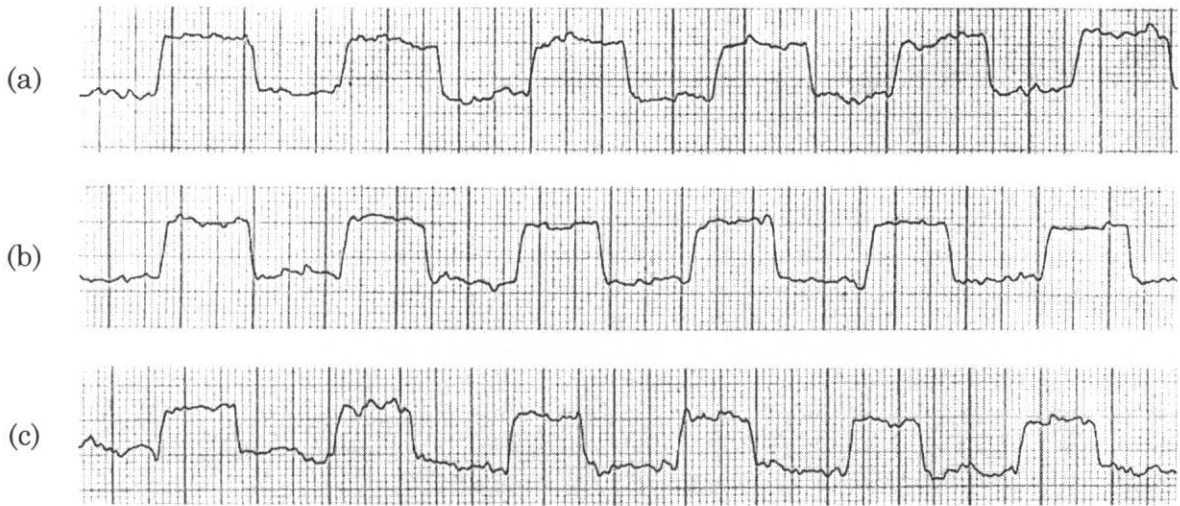
Fig. 3-8. Groove profiles of the present holographic grating measured by a contact probe at (a) w = +35 mm, (b) w = 0 mm and (c) w = -35 mm.
