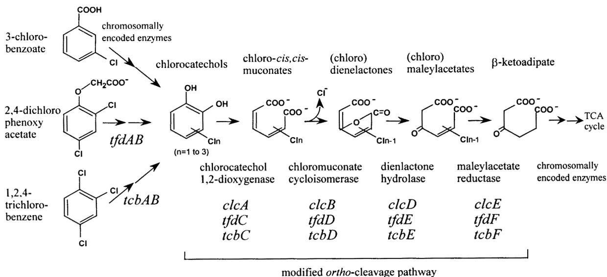
Fig. 1. Pathways for degradation of chlorinated aromatic compounds via modified *ortho*-cleavage pathway.
