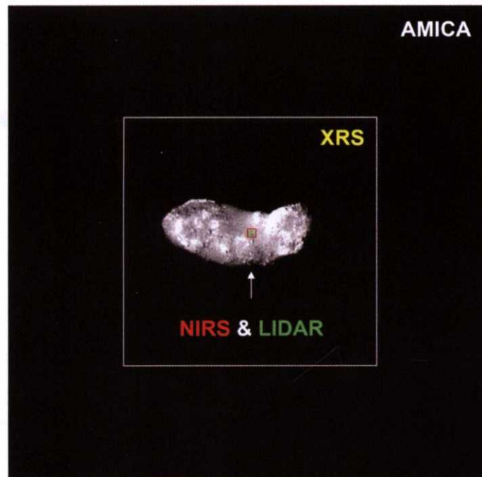
Figure 4-2-1 : Field of view of each instrument (AMICA 5.7x5.7deg, XRS 3.0 x 3.0deg, NIRS 0.1x 0.1deg, LIDAR 0.04 x 0.097deg).
