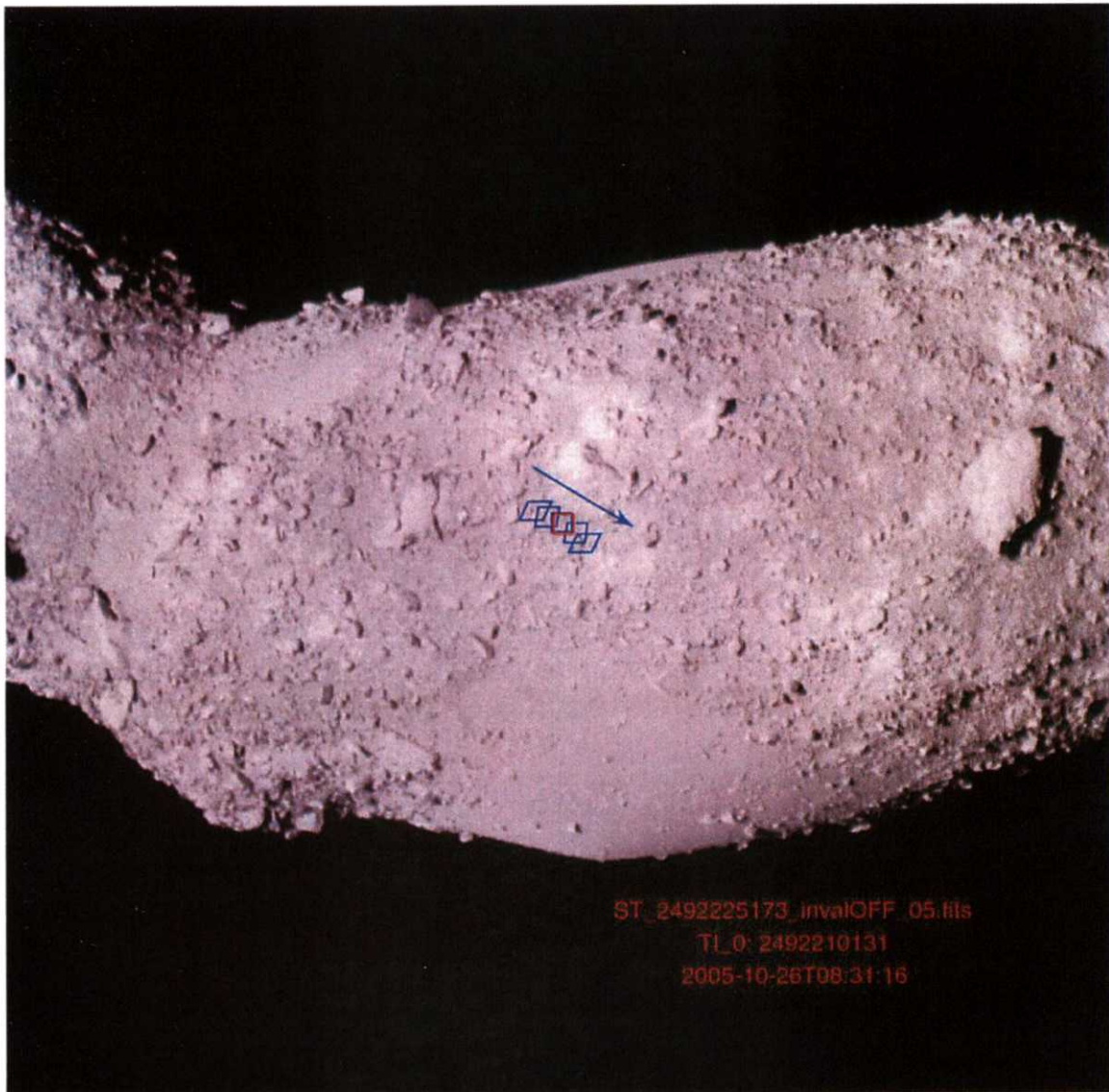
Figure 5-5-2: Footprint for observing the boulder-rich area (Figure 5-5-1) is denoted by a small red square. Blue square is footprints for observing its neighborhood (Figure 5-5-5). An arrow is the move direction of the NIRS footprint. Image data is obtained by AMICA (ST_249225173).
