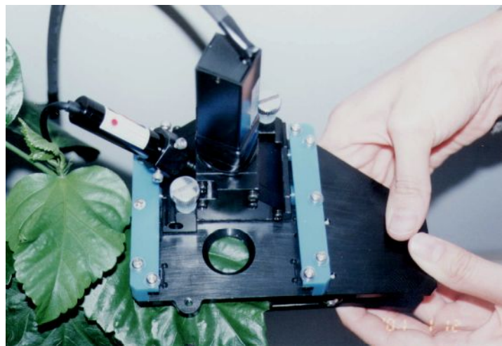
Fig. 4.13 The leaf folder set to a leaf. After setting a cover is slid to make dark adaptation of the leaf.
