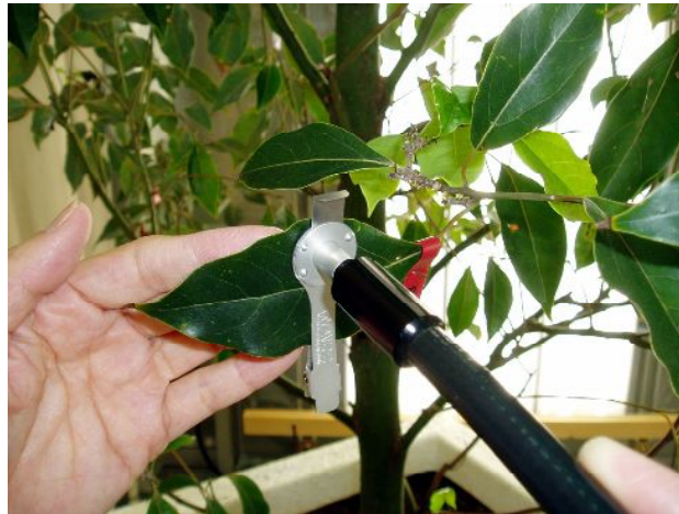
Fig. 4.20 Measuring fluorescence using Dias II (close up). Laser is irradiated and fluorescence is measured, after setting the optical fiber to a leaf clip.
