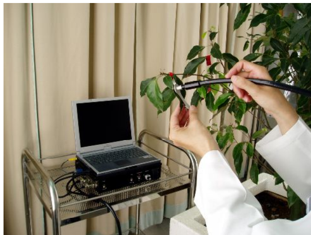
Fig. 4.21 Measuring fluorescence using Dias II .
