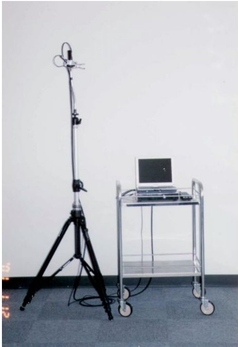
Fig. 4.7 Whole view of Dias I . Left: leaf folder attached to the tripod, Right: console box and PC.
