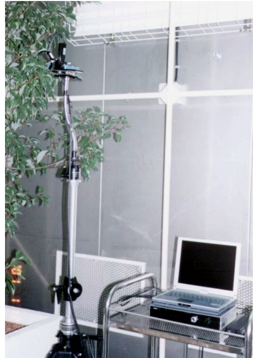
Fig. 4.8 Measuring fluorescence using Dias I . It can measure to a height of 3 m.
