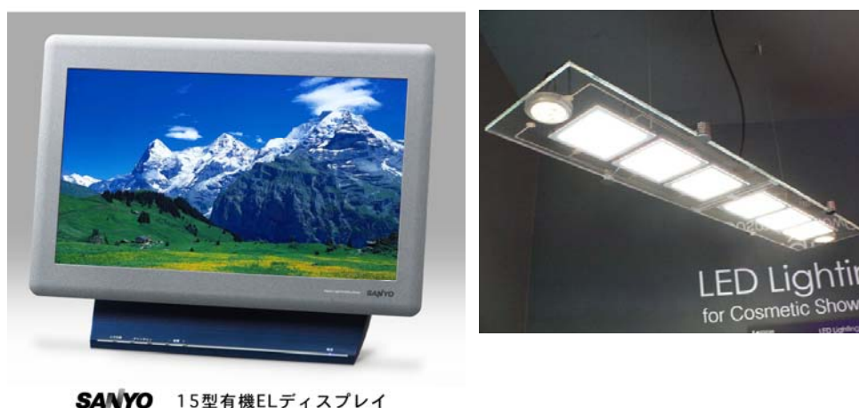
Figure 1-15. Left: SANYO 15" active-matrix full-color display with white OLEDs and color filters demonstrated at CEATEC in October 2002. Right: OLED light demonstrated by Koizumi in 2003
