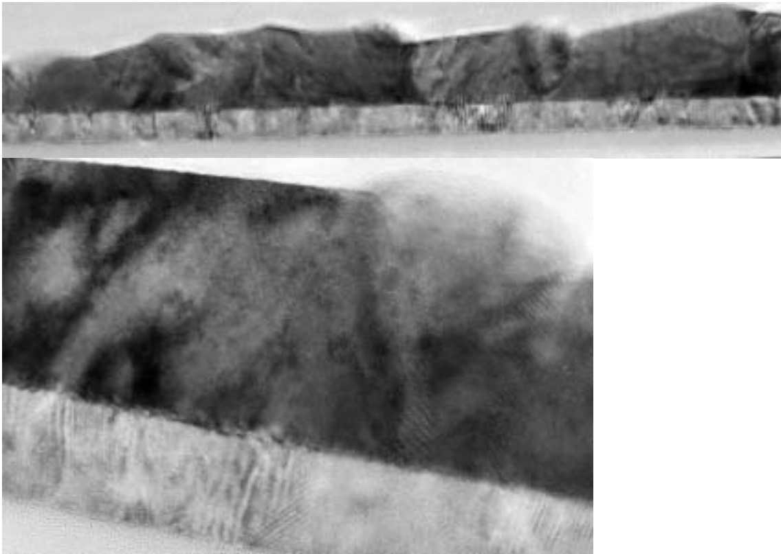
Fig. 3-3-19. Cross-sectional TEM images of FePt/TiN monolayer system for various t_{\text{FePt}} . The deposition condition of each layer is the same as samples shown in fig. 3-2-18.
