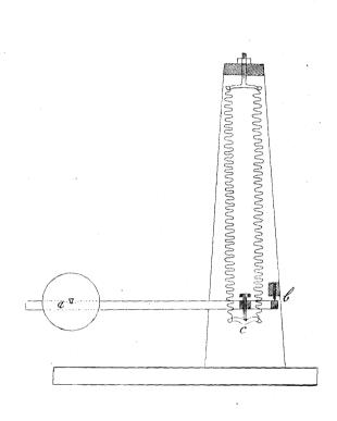
placed that when the weight goes down\* the fluid runs over towards it and increases the weight, and vice versa.
