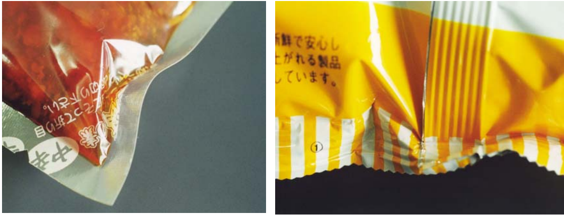
Photo 6-3 Tuck which arose in packaged goods
