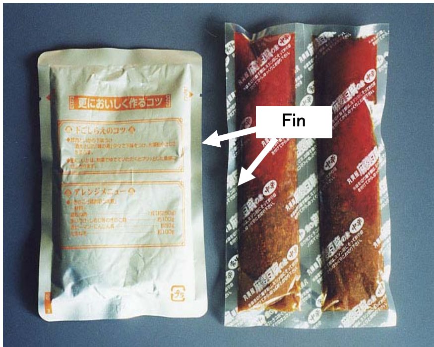
Photo 7-1 Heat sealing Fin of the flexible packaging
