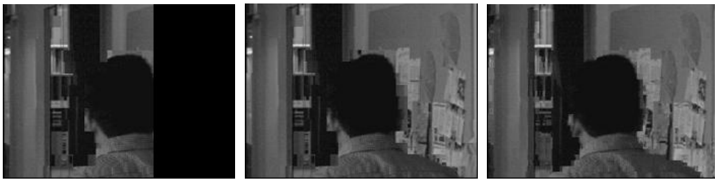
(a) 16x16pel 片方向予測 (b) 16x16pel 双方向予測 (c) 8x8pel 双方向予測 12.23dB(4.06bit/block) 26.62dB(5.71bit/block) 29.03dB(6.45bit/block)
