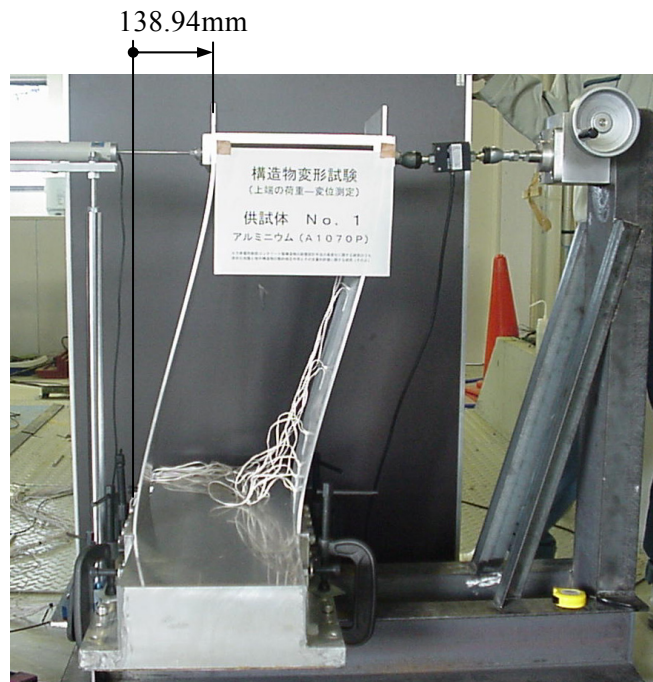
Photo.2.8: Structure model with the maximum displacement (Structure-B, A1070P)
