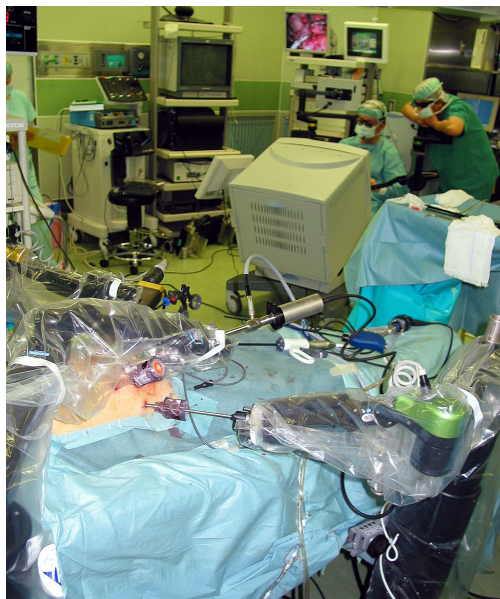
Fig.6.11 Scene of ZEUS surgery at Kyushu university hospital and link mechanism of ZEUS manipulator
