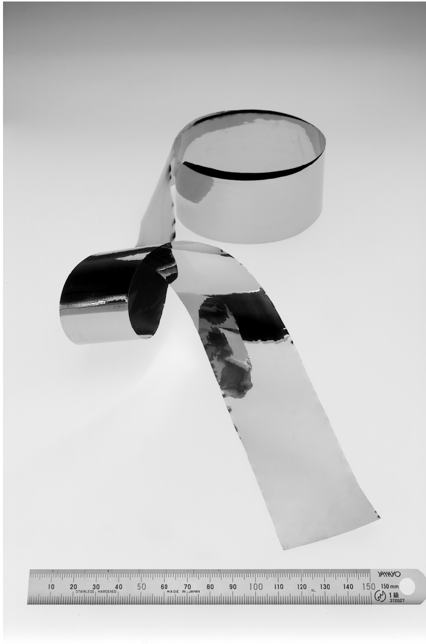
図 4.4: A heavily cold-rolled \text{Ni}_3\text{Al} foil of sample DS24-47 (Investment-Cast materials) with 99% reduction in thickness. The dimensions of the foil are 23\ \mu\text{m} in thickness, 50 mm in width, and 650 mm in length.
