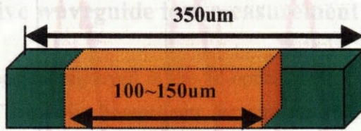
Fig.5.8 Schematic module for the measurement of the coupling loss at the butt joint interface.
