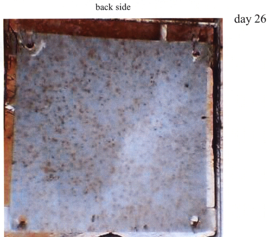
Figure 3-4. Surface conditions of test panel after 26 days in Tokyo bay (1).
