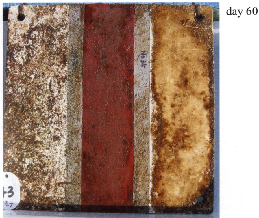
Figure 3-2. Surface conditions of test panel after 30 days and 60 days in Shizugawa bay (1).
