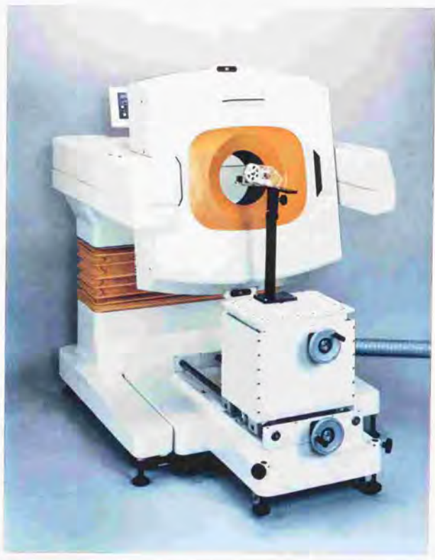
Fig.4-2 External view of gantry/detector unit
