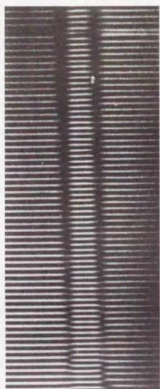
Fig. 4-12 An example of an interference pattern obtained with the cell shown in Fig. 4-11. The refractive index of the liquid sample in the cell was determined by measuring the interval of the fringes. The center part of the image was due to the acrylic partition. Both sides fringes were caused by the samples.
