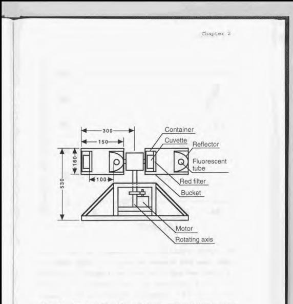
Fig. 2 The centrifugation equipment. The electric power for the light source for each bucket was supplied via the rotating axis. At maximum rotation (260 rpm), the protonemata were exposed to basipetal hypergravity at  $20 \times g$ (Basi-20×g) or acropetal hypergravity at  $13 \times g$  (Acro- $13 \times g$ ). Numbers refer to distances in mm.
