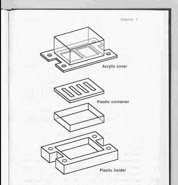
Fig. 1 The attachment for the centrifugation system. A plastic container was stuffed with rock wool and filled with agar medium. Assembled attachment was bolted to the bucket and centrifuged. White light was irradiated from above in this figure.
