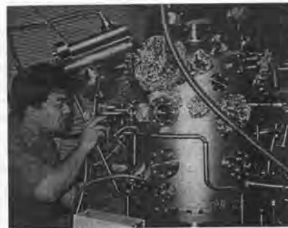
FIG. 2.6. Photograph of our PES apparatus. The electron energy analyzer (VG Microtech, CLAM-II), which is seen above the head of the author, are equipped on the "Mu-metal" UHV chamber. The Mg K \alpha x-ray source and the He discharge lamp are equipped below the CLAM-II analyzer.
