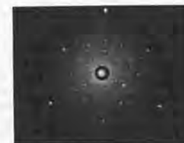
FIG. 4.8. Laue photographs of the single-crystalline \text{SrVO}_3 at room temperature. See text for details.
