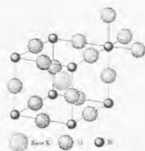
Figure 5.1: Basic crystal structure of BKBO is, i. e., the three-dimensional perovskite structure. The BiO_6 octahedra are tilted and shows breathing for x < x_c .
