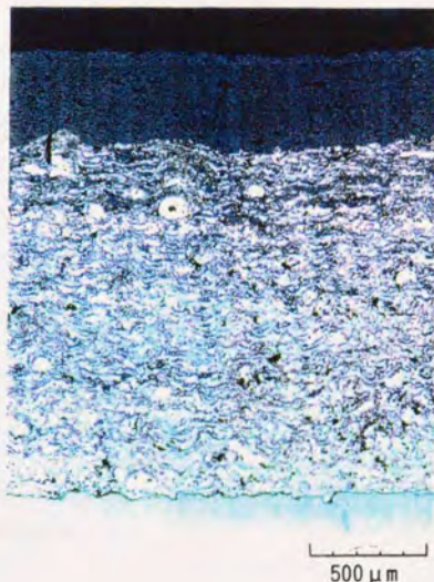
Fig. 5-13 Microstructure of graded sprayed coating of cylinder head after engine test
