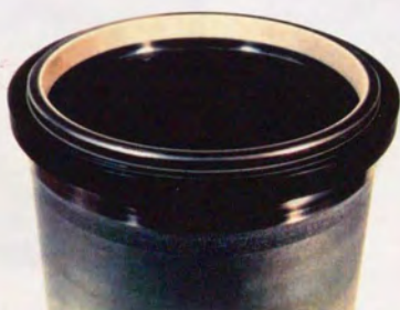
Fig.5-11 Appearance of ceramic sprayed cylinder liner
