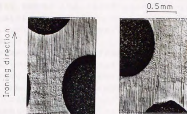
Fig.6 Infiltration of less viscous lubricant into boundary contact region under processing ( L: 0.5mm, Lubricant: Ip ).
