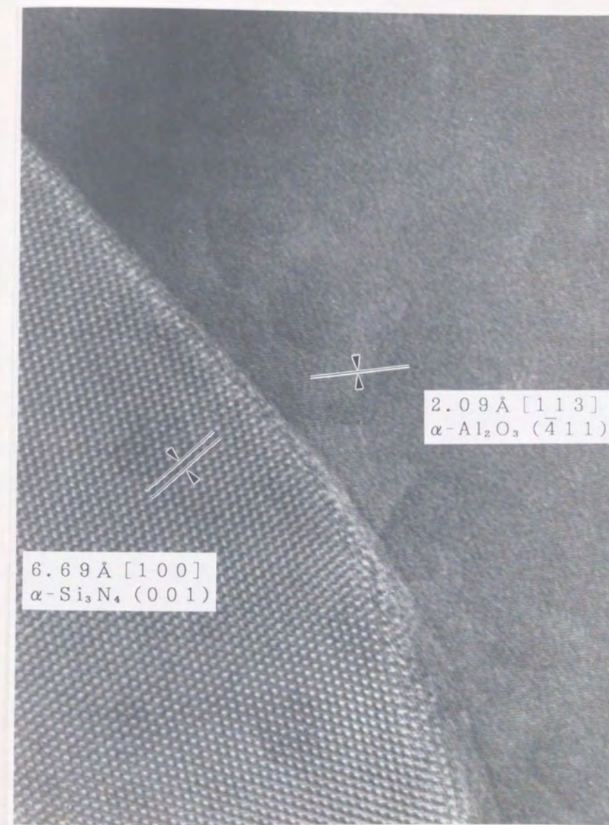
Fig.5.10 High resolution TEM image showing interface between Al 2 O 3 and Si 3 N 4 in the sintered body
