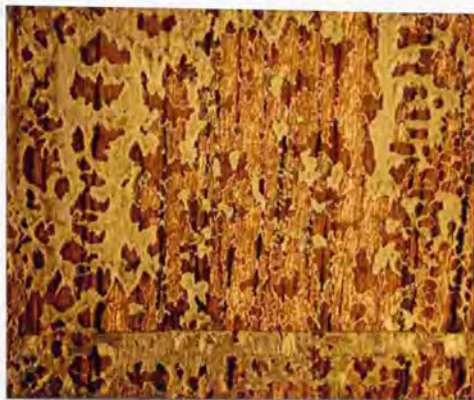
Fig. 15. Photograph of the fractured surface for a block-shear specimen. Notes: Bond strength of this specimen was 50.3 \text{ kgf/cm}^2 and the effective glue-spreading area was relatively wide.
