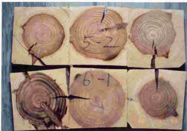
Fig. 26. Delamination of joints after drying.
