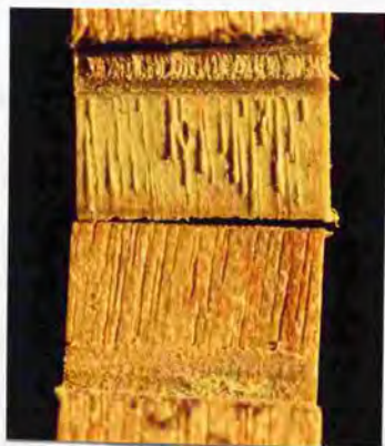
Fig. 9. A uniform glue line obtained by a pressure of 0.2 kgf/cm 2 for 24 hrs.
