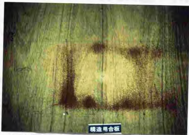
Fig. 81. Chladni pattern of full-sized floor.
