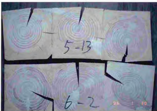
Fig. 27. Delamination of coated joints after drying.
