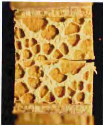
Fig. 10. A thick and net-shaped glue line resulting from spacers.
