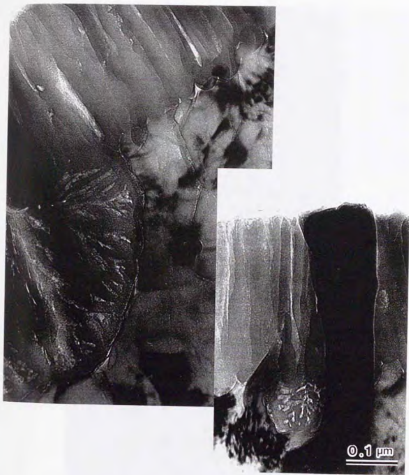
Fig.3.3.4 Electron micrographs of the ultramicrotomed sections of the anodic films during current recovery by sudden voltage drop from 40 V to 20 V.
