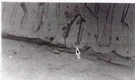
Fig.3.2.7 Electron micrographs of the section of anodic films formed in Ematal bath at 120 V for 10 min. An arrow indicates voids in the barrier layer.
