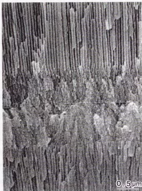
Fig.6.6 SEM image of a fracture section of a film formed as a membrane having center-minuteness. Forming condition ; 0.3 \text{ mol dm}^{-3} oxalic acid at 30 V for 1 h, 10 V for 20 min, suddenly drop to 5 V, kept for 1 h, 10 V for 20 min, 30 V for 1 h, decreased to 1 V.
