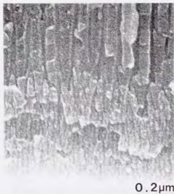
Fig.6.8 SEM image of a film ( near barrier layer ) formed as a membrane having both side minuteness. Forming condition ; 0.15 \text{ mol dm}^{-3} ammonium tartrate at 10 V for 5 min, subsequently re-anodized in 0.3 \text{ mol dm}^{-3} oxalic acid at 10 V for 10 min, 40 V for 2 h, 10 V for 10 min, decreased to 2 V.
