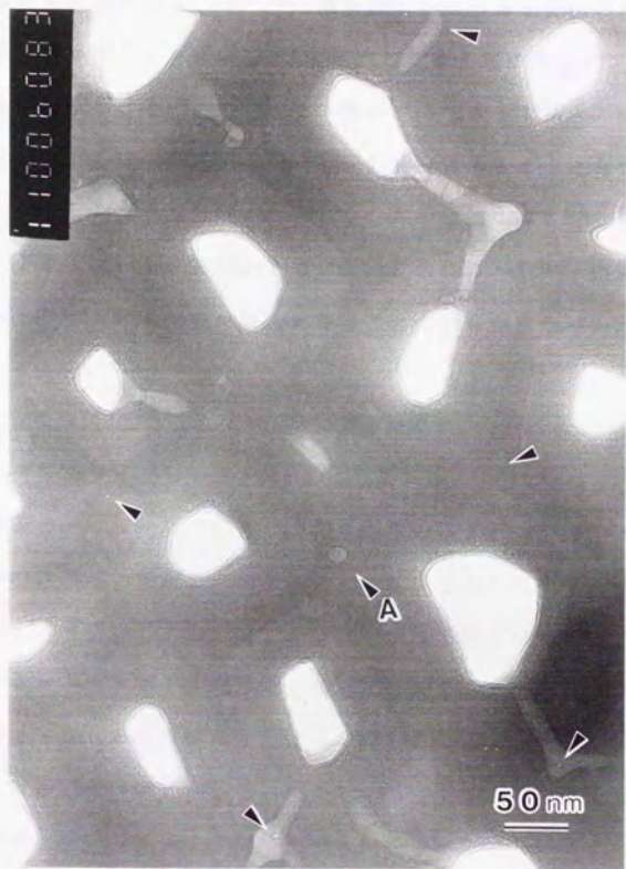
Fig.4.1.6 TEM image of an ion-thinned anodic film formed in a 0.4 mol \text{dm}^{-3} phosphoric acid solution (25°C) at 80 V for 5 min. Arrow A indicates a void including an oxide particle. Other arrows indicate fine voids with the diameter of 2-3 nm at triple cell junctions.
