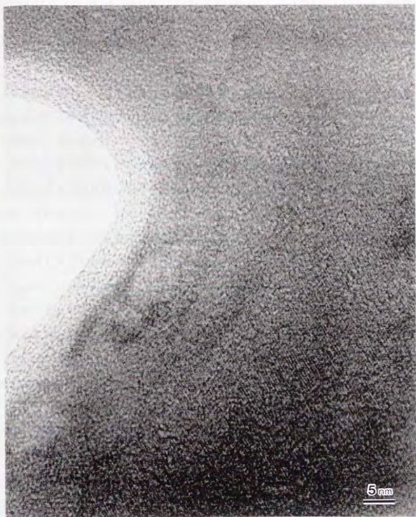
Fig.5.2.7 High resolution images of crystallized anodic film formed in phosphoric acid solution at 80 V for 5 min after exposure to the electron beam.
