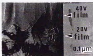
Fig.6.2 TEM image of the ultramicrotomed section of an anodic film formed in 0.3 mol \text{dm}^{-3} oxalic acid ( 30^{\circ}\text{C} ) at 40 V and suddenly dropped to 20 V and kept until early period of current recovery.
