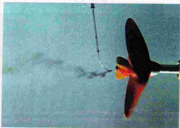
Fig. 2-4 Hub Vortex Visualized by Dye Injection Method
