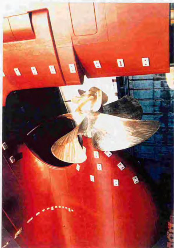
Fig. 7-1 PBCF Installation on "Mercury Ace"
