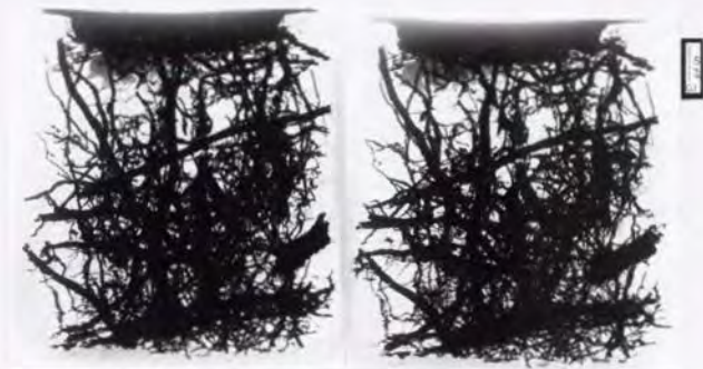
写真Ⅲ-4 岩手ローム、限界間隙を含む粗孔隙像 (写真3と同じ試料) Iwate loam, Undist. soil, Coarse pores with Entry pore (Sample is the same as Photo. 3 sample)
