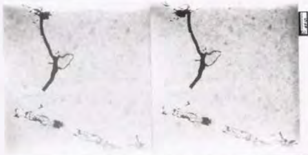
写真Ⅲ-1 岩手ローム、自然構造、貫通開放孔隙 Iwate loam, Undist. soil, A pore completed air penetration over sample length
