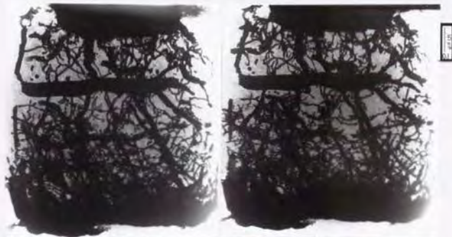
写真Ⅲ-8 安達太良ローム、限界間隙を含む粗孔隙像 (写真7と同じ試料) Adataro loam, Undist. soil, Coarse pores with Entry pore (Sample is the same as Photo. 7 sample)
