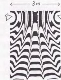
Fig.4.6 Contours of constant group delay for L=R (freq: 500Hz, sound velocity: 341m/s, free field, omni-directional loudspeakers). The black and white areas appear alternately at intervals of 0.5ms.
