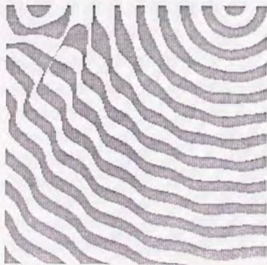
Fig.4.4 Contours of constant phase for L=0.3e^{j0.95\pi}R (freq:500Hz, sound velocity: 341m/s, free field, omnidirectional loudspeakers). The black and white areas appear alternately at intervals of \pi/4 .
