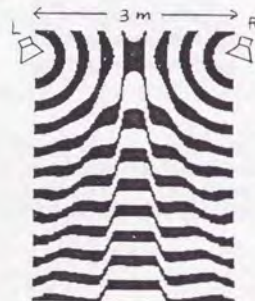
Fig.4.7 Contours of constant time delay by cross-correlation for L=R (freq:500Hz, sound velocity: 341m/s, free field, omni-directional loudspeakers). The black and white areas appear alternately at intervals of 0.5ms.
