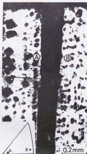
Fig.7-6 Intergranular cracking and orientation of grain boundary plan ( \theta = 90^\circ ).
