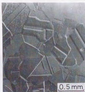
Fig.8-4 Steps formed by potentiostatic etching for commercial Alloy 600 polycrystals.
