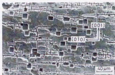
Fig.5-11 Transgranular cacks propagating along \{100\} traces on the surface.
