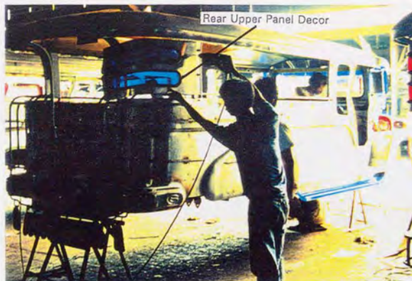
The decorations for the body shell are installed.
