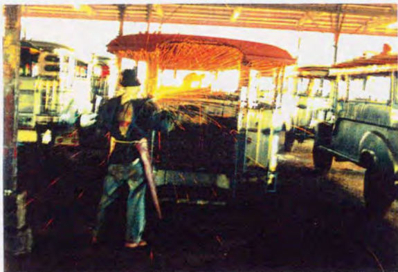
Metal finishing process using a grinder machine.
