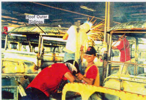
The roof outer sidings are made up of angle bar and strip of stainless steel metal sheet.
