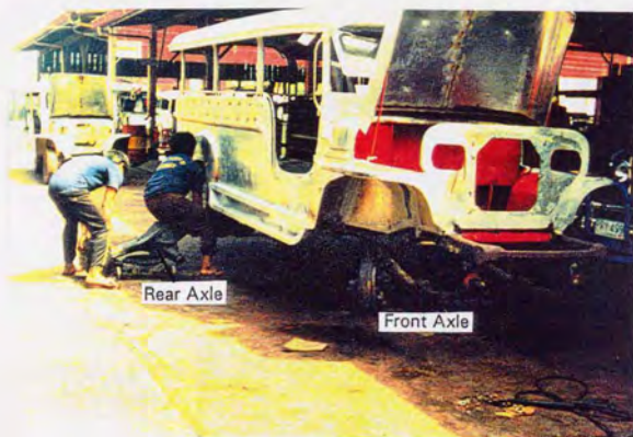
The front axle and rear axle are installed.
