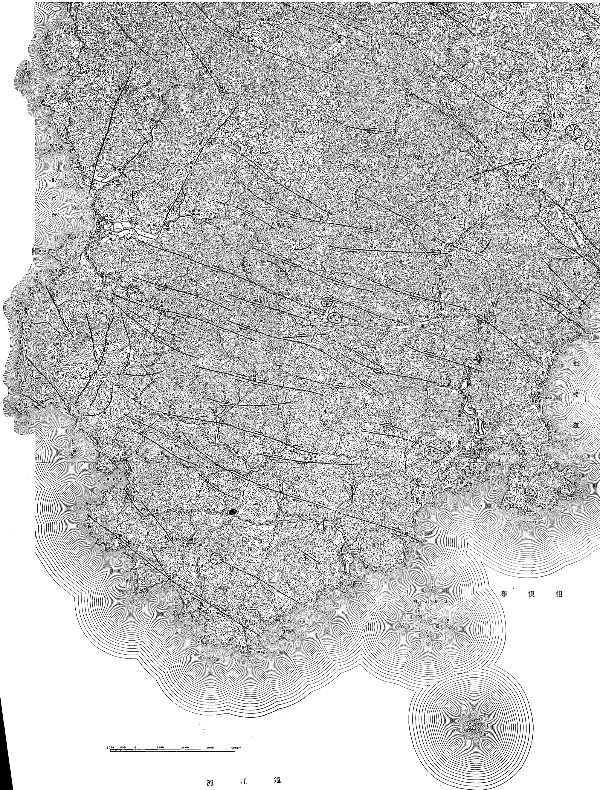
Fig. 96. Active faults and lineaments in the southern end of the Izu Peninsula.
