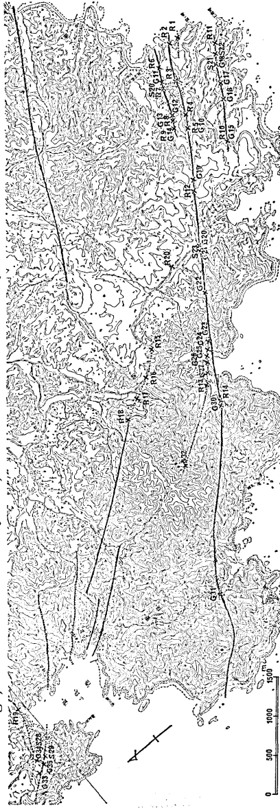
Fig. 14-2. A map showing the locations of outcrops, surface cracks, and fissures and damaged houses, on the earthquake faults and the active faults.
