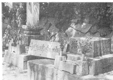
Fig. 10. Rotation and overturning of gravestones at Shimoda (Kaizen-ji).
