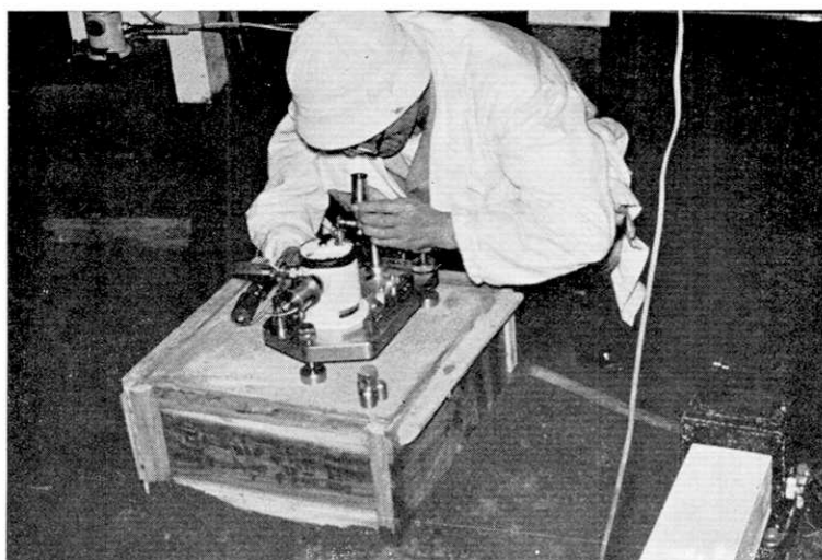
Fig. 1.4. A portable water-tube tiltmeter (test observation at Aburatsubo).
