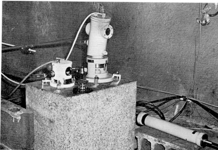
Fig. 2.5. Comparison of an ultrasonic water-tube tiltmeter (right) with a manual reading water-tube tiltmeter (left).
