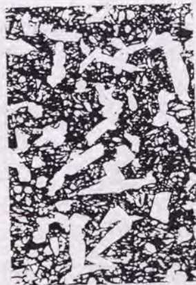
d) P4 : White precipitates; (Fe,Cr)_7C_3 Matrix : Martensite
