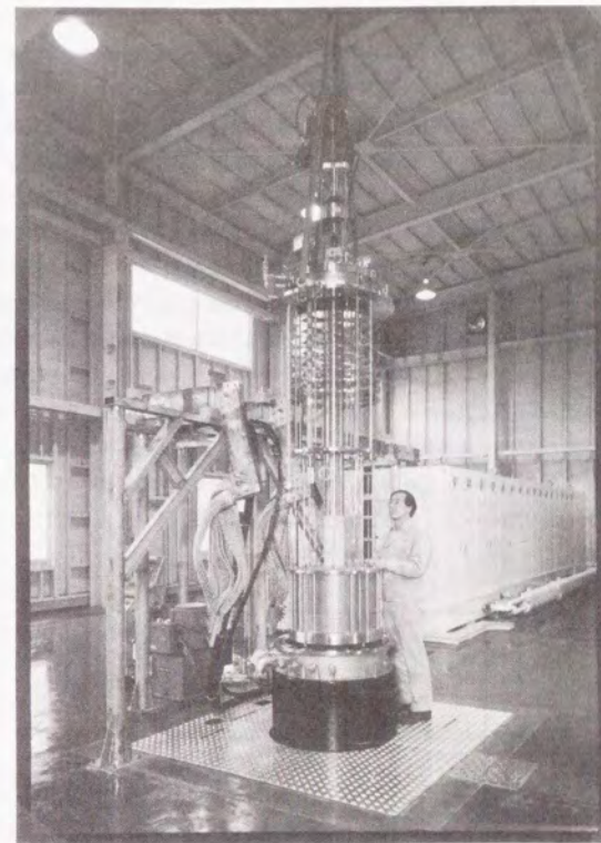
写真5.7 応力下超電導体試験装置の超電導マグネットを引き上げた状態 Photo 5.7 The appearance of superconducting magnets and others of the test facility.
