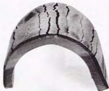
(b) A5052+<A5056(#32)+WA(#1500), V_p=20\% > P=88\text{MPa} T=614^\circ\text{C} , \phi=70\% (A5056), \phi=93\% (A5052)
