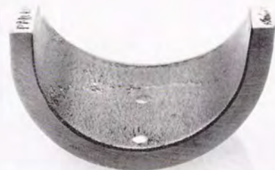
(a) A5052+<A5056(#32)+WA(#1500), V_p=20\% > P=49\text{MPa} T=615^\circ\text{C} , \phi=70\% (A5056), \phi=92\% (A5052)
