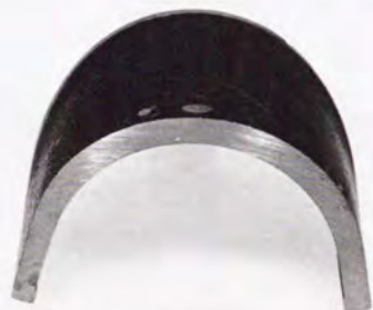
(c) A5052+<WA(#1500)> P=127\text{MPa} T=615^\circ\text{C} , \phi=92\% (A5052)
