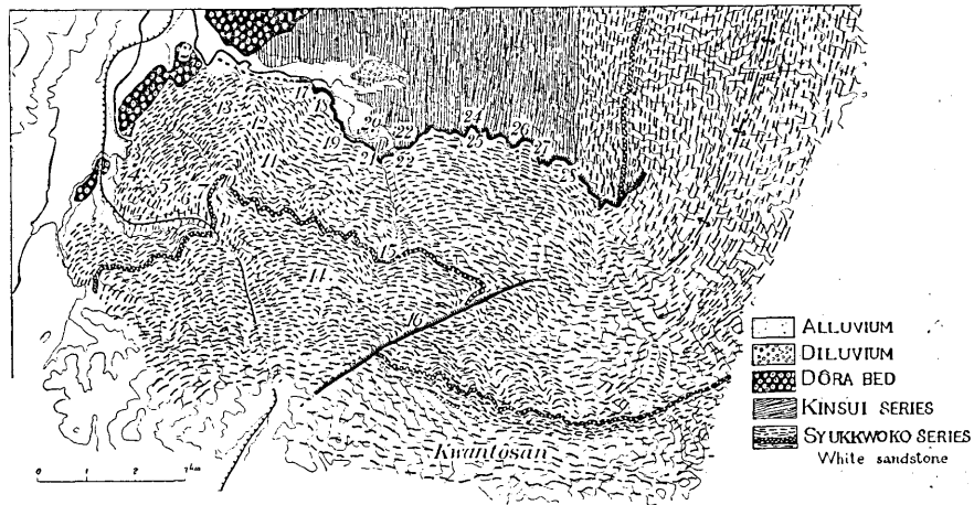
第7圖 關刀山附近の地質圖。三叉逆斷層を示す。 Geologic map near Mt. Kwantō (-san). Numerals show the localities of exposure referred in this paper.
