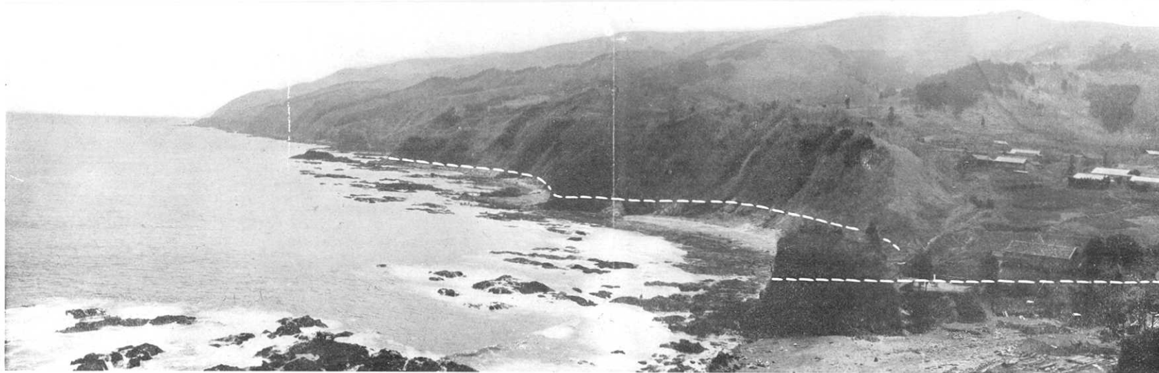
第 310 圖 綾里村野々前附近より綾里岬を望む. 圖中點線は津浪の到達せる最高所の跡を示めしてをり圖に矢をもつてその附近の浪高を示めず. 綾里灣口より灣奥に入るに従ひ浪高の高くなるのが見られる. (4 月 5 日 西村, 高山撮影) Fig. 310. Ryori cape as seen from near Nonomae, Ryori village. Dotted line shows maximum heights reached by tsunami; the same for particular points indicated by arrows. It will be seen that the wave heights increase with distance from the mouth of the bay landwards. (Photo by G. Nishimura and T. Takayama, April 5.)
