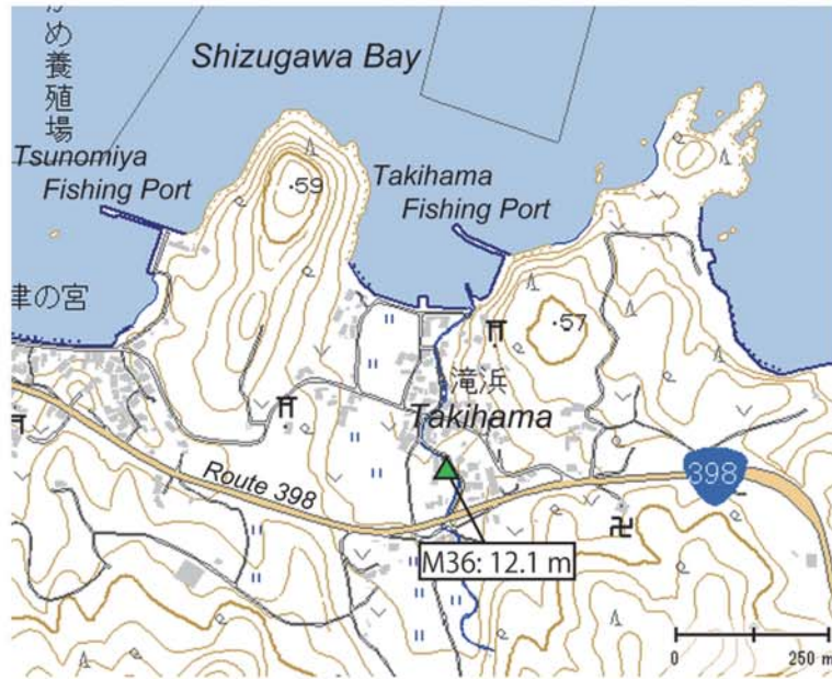
Fig. A175. Tsunami height at Takihaman, Tokura, Minamisanriku Town, Miyagi Prefecture (added with a digital topographic map at a scale of 1/25,000 from the Geospatial Information Authority of Japan). The symbol and its meaning are the same as in Fig. 4.
