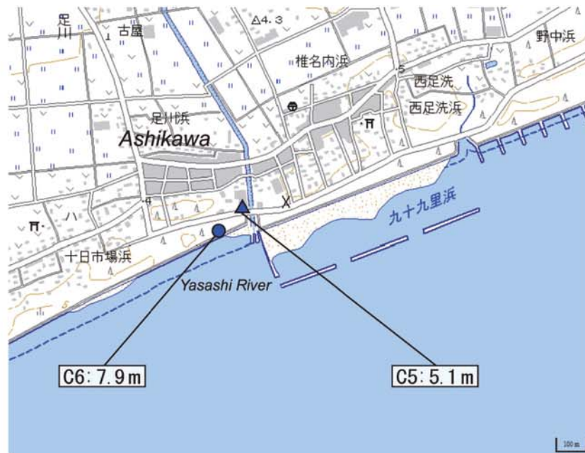
Fig. A299. Tsunami heights at Ashikawa, Asahi City, Chiba Prefecture (added with a digital topographic map at a scale of 1/25,000 from the Geospatial Information Authority of Japan). The symbols and their meanings are the same as in Fig. 6.
