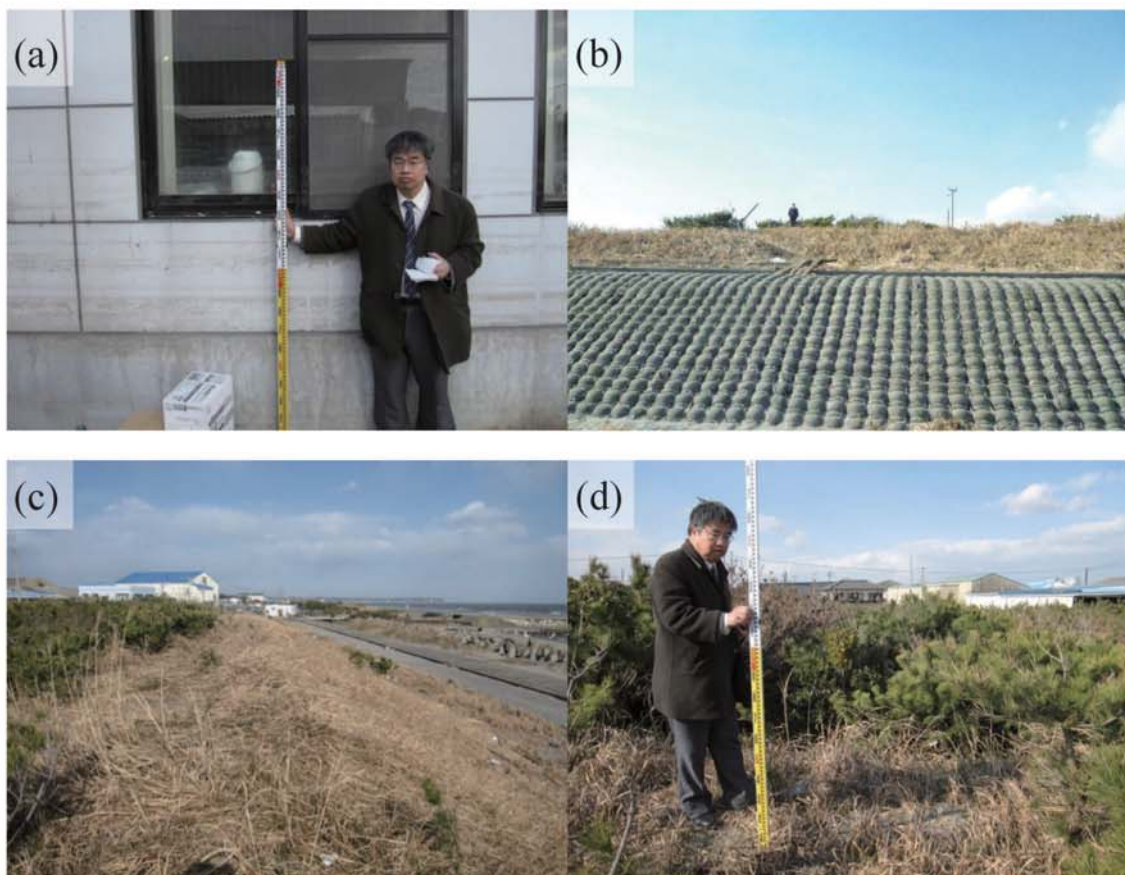
Fig. A300. (a) Watermark on a wall of a fish-processing factory (1.655 m above ground level; C5). (b)-(d) Tsunami inundated a sanddune near the Yasashi River (C6).
