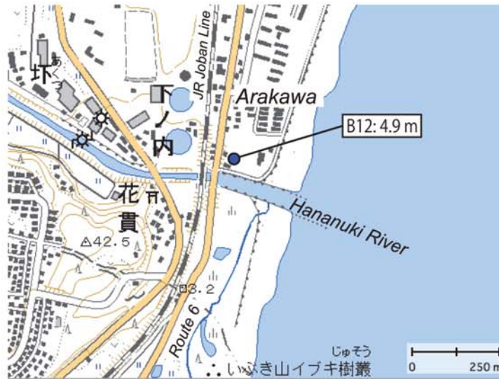
Fig. A253. Tsunami height at Arakawa, Takahagi City, Ibaraki Prefecture (added with a digital topographic map at a scale of 1/25,000 from the Geospatial Information Authority of Japan). The symbol and its meaning are the same as in Fig. 5.
