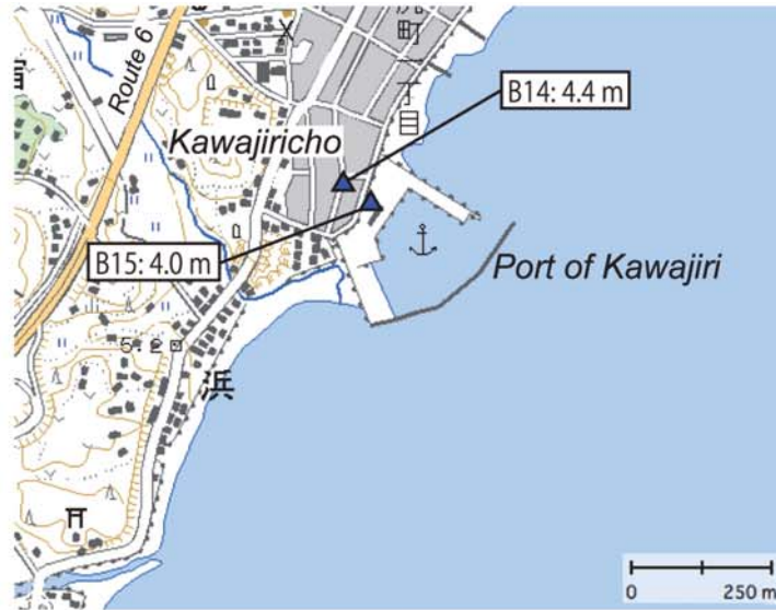
Fig. A257. Tsunami heights at Kawajiricho (Port of Kawajiri), Hitachi City, Ibaraki Prefecture (added with a digital topographic map at a scale of 1/25,000 from the Geospatial Information Authority of Japan). The symbols and their meanings are the same as in Fig. 5.
