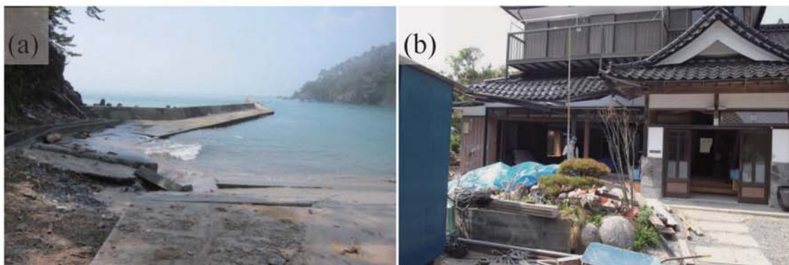
Fig. A140. (a) Damage at Karakuwacho-Tsumoto. (b) Tsunami trace survey point at the drying area on the second floor (4.70 m above ground level, M4).
