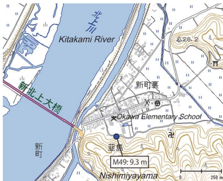
Fig. A191. Tsunami height at Nishimiyayama, Kamaya, Ishinomaki City, Miyagi Prefecture (added with a digital topographic map at a scale of 1/25,000 from the Geospatial Information Authority of Japan). The symbol and its meaning are the same as in Fig. 4.
