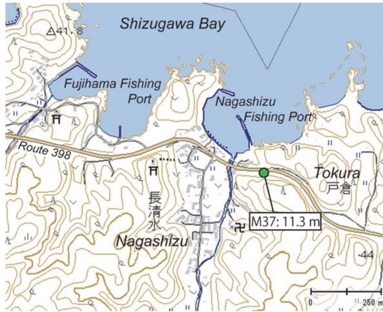
Fig. A177. Tsunami height at Nagashizu, Tokura, Minamisanriku Town, Miyagi Prefecture (added with a digital topographic map at a scale of 1/25,000 from the Geospatial Information Authority of Japan). The symbol and its meaning are the same as in Fig. 4.
