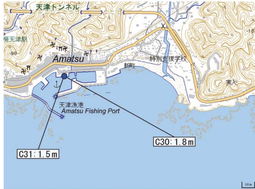
Fig. A335. Tsunami heights at Amatsu (Amatsu Fishing Port), Kamogawa City, Chiba Prefecture (added with a digital topographic map at a scale of 1/25,000 from the Geospatial Information Authority of Japan). The symbols and their meanings are the same as in Fig. 6.
