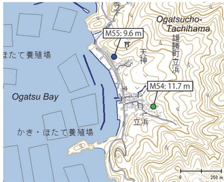
Fig. A201. Tsunami heights at Ogatsucho-Tachihama, Ishinomaki City, Miyagi Prefecture (added with a digital topographic map at a scale of 1/25,000 from the Geospatial Information Authority of Japan). The symbols and their meanings are the same as in Fig. 4.
