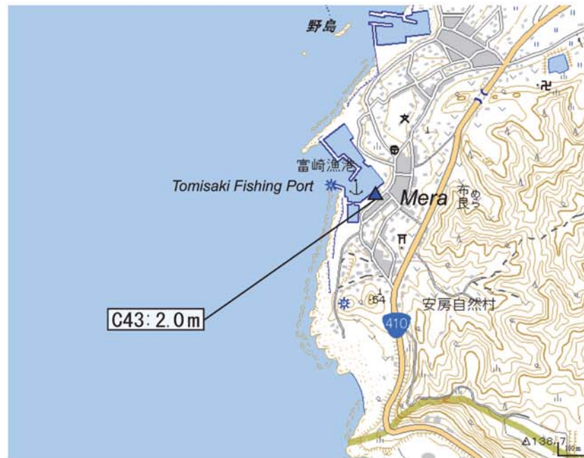
Fig. A353. Tsunami height at Mera (Tomisaki Fishing Port), Tateyama City, Chiba Prefecture (added with a digital topographic map at a scale of 1/25,000 from the Geospatial Information Authority of Japan). The symbol and its meaning are the same as in Fig. 6.
