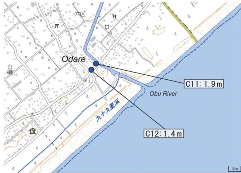
Fig. A307. Tsunami heights at Odare, Yokoshibahikari Town, Chiba Prefecture (added with a digital topographic map at a scale of 1/25,000 from the Geospatial Information Authority of Japan). The symbols and their meanings are the same as in Fig. 6.
