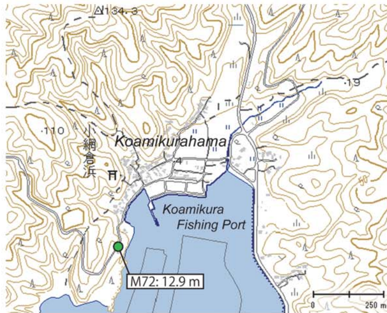
Fig. A229. Tsunami height at Koamikurahama, Ishinomaki City, Miyagi Prefecture (added with a digital topographic map at a scale of 1/25,000 from the Geospatial Information Authority of Japan). The symbol and its meaning are the same as in Fig. 4.
