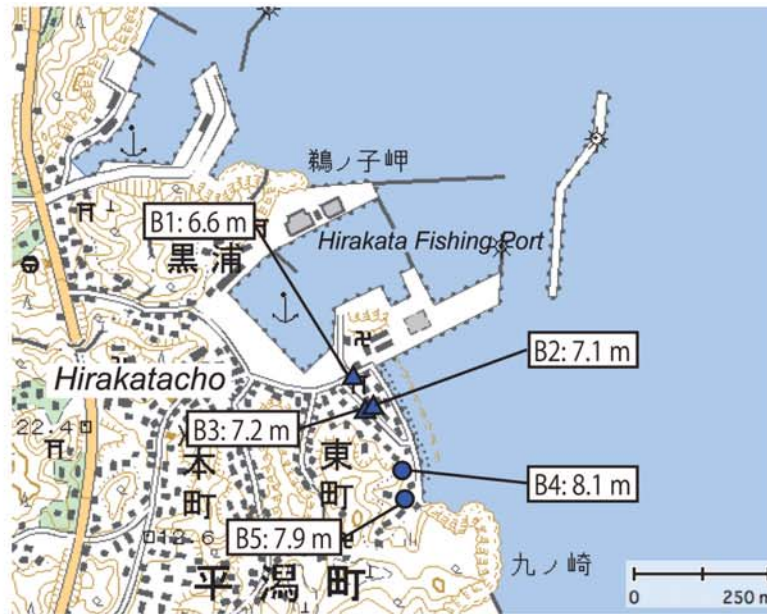
Fig. A239. Tsunami heights at Hirakatacho, Kitaibaraki City, Ibaraki Prefecture (added with a digital topographic map at a scale of 1/25,000 from the Geospatial Information Authority of Japan). The symbols and their meanings are the same as in Fig. 5.
