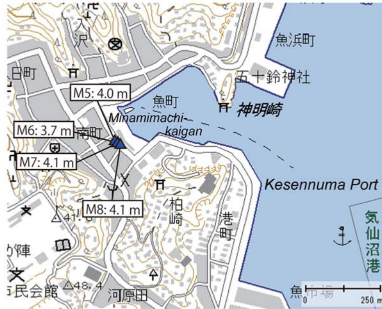
Fig. A141. Tsunami heights at Minamimachikaigan (Kesennuma Port), Kesennuma City, Miyagi Prefecture (added with a digital topographic map at a scale of 1/25,000 from the Geospatial Information Authority of Japan). The symbols and their meanings are the same as in Fig. 4.
