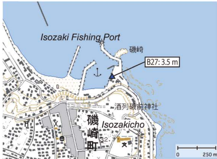
Fig. A277. Tsunami height at Isozakicho (Isozaki Fishing Port), Hitachinaka City, Ibaraki Prefecture (added with a digital topographic map at a scale of 1/25,000 from the Geospatial Information Authority of Japan). The symbol and its meaning are the same as in Fig. 5.
