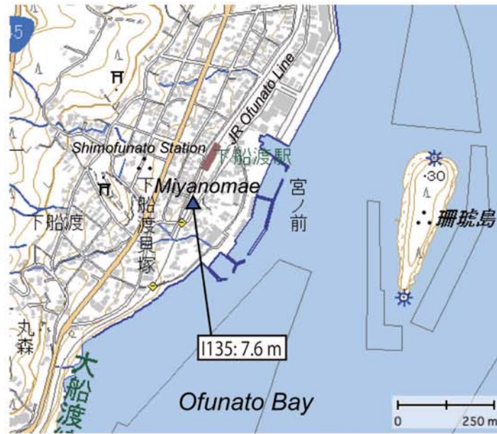
Fig. A129. Tsunami height at Miyanomae, Ofunatocho, Ofunato City, Iwate Prefecture (added with digital topographic map at a scale of 1/25,000 from the Geospatial Information Authority of Japan). The symbol and its meaning are the same as in Fig. 4.
