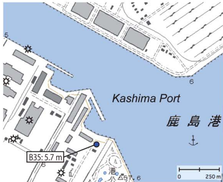
Fig. A287. Tsunami height at Higashifukashiba (Kashima Port), Kamisu City, Ibaraki Prefecture (added with a digital topographic map at a scale of 1/25,000 from the Geospatial Information Authority of Japan). The symbol and its meaning are the same as in Fig. 5.
