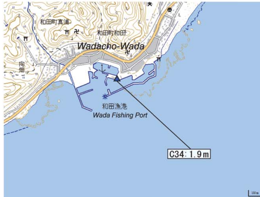
Fig. A341. Tsunami height at Wadacho-Wada (Wada Fishing Port), Minamiboso City, Chiba Prefecture (added with a digital topographic map at a scale of 1/25,000 from the Geospatial Information Authority of Japan). The symbol and its meaning are the same as in Fig. 6.
