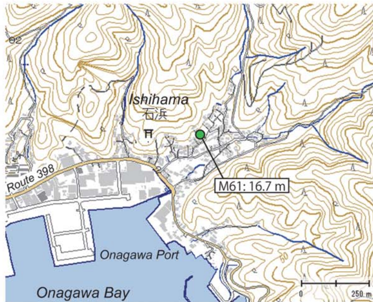
Fig. A213. Tsunami height at Ishihama, Onagawa Town, Miyagi Prefecture (added with a digital topographic map at a scale of 1/25,000 from the Geospatial Information Authority of Japan). The symbol and its meaning are the same as in Fig. 4.
