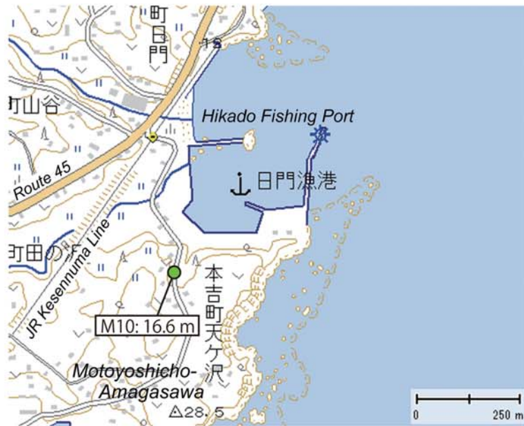
Fig. A145. Tsunami height at Motoyoshicho-Amagasawa (Hikado Fishing Port), Kesennuma City, Miyagi Prefecture (added with a digital topographic map at a scale of 1/25,000 from the Geospatial Information Authority of Japan). The symbol and its meaning are the same as in Fig. 4.
