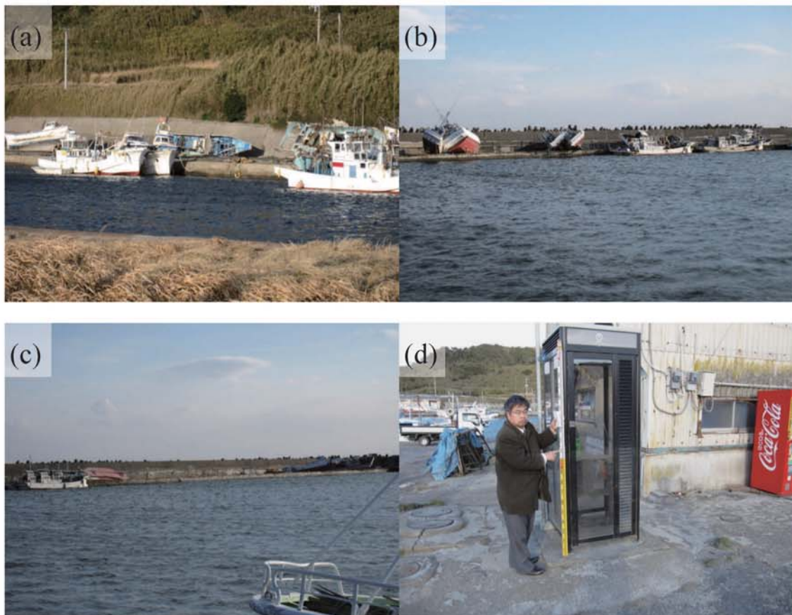
Fig. A296. (a)-(c) Damage at Iioka Fishing Port. (d) Watermark on the wall of a telephone box in Iioka Fishing Port (1.07 m above ground level; C3).
