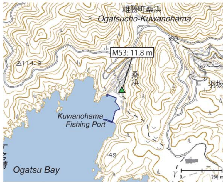
Fig. A199. Tsunami height at Ogatsuchō-Kuwanohama, Ishinomaki City, Miyagi Prefecture (added with a digital topographic map at a scale of 1/25,000 from the Geospatial Information Authority of Japan). The symbol and its meaning are the same as in Fig. 4.
