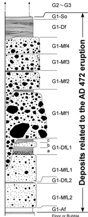
Fig. 4. Model column of deposits related to the 472 eruption of Vesuvius volcano in areas excavated in 2006–2008. Mf means massive, matrix-supported debris flow facies. Df means stratified, clast-supported debris flow facies. G1-Mf1 directly covers G1-Af in a southern area.
