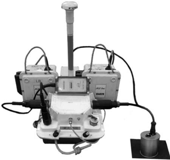
Fig. 6. Outlook of earthquake observation system employed with analog-output type MEMS accelerometer sensor.
