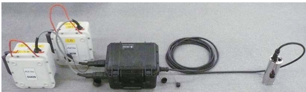
Fig. 8. Outlook of earthquake observation system employed with digital-output type MEMS accelerometer sensor.
