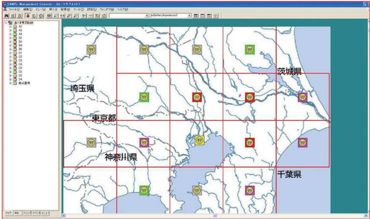
Fig. 2. Screen shot of Simple Network Management Protocol (SNMP) monitoring window. The colors of icons change from green to red through yellow and pink as the degree of the problem is increased.
