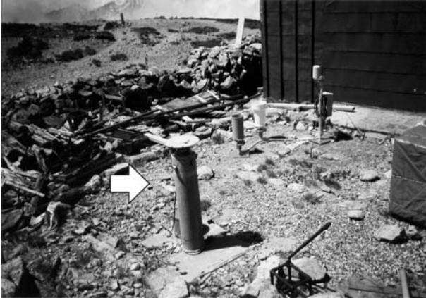
Fig. 2. Jododaira station for GPS observation. Arrow indicates the concrete pillar and GPS antenna. The wall at the back of photo is Tateyama Laboratory, University of Toyama.
