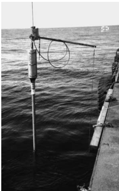
Fig. 1. Photograph of a piston corer used for sediment sampling.
