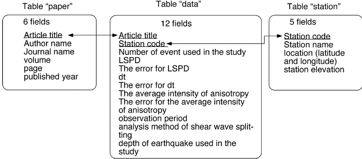
Fig. 3. The structure of tables used in the present system. Each table can be related to other tables (allowed in the figure) using “key” in each table (underlined).
