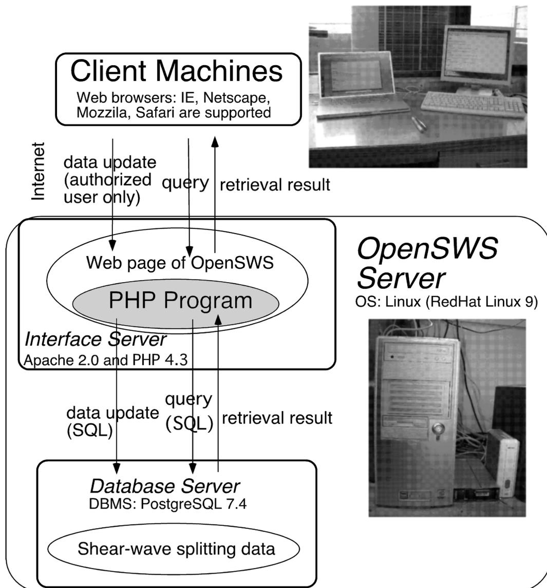
Fig. 2. Block diagram of the database system, OpenSWS. This system provides all of the services on the web page with the interface server.
